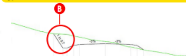
Figure 15: Typical cross-section through the Access Road where there is a section of cut and fill. Shown in Chainage 1100.
