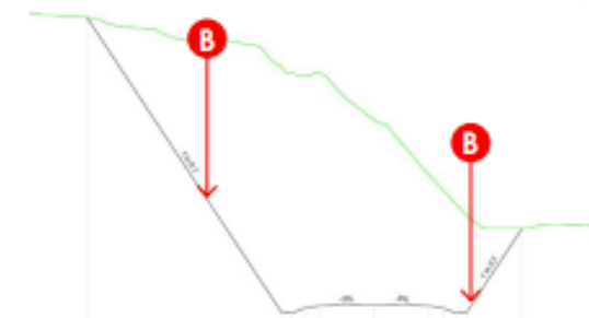
Figure 14: Cross-section through the Access Road at Granite Creek, which has a significant cut. Chainage 1500 is shown.
