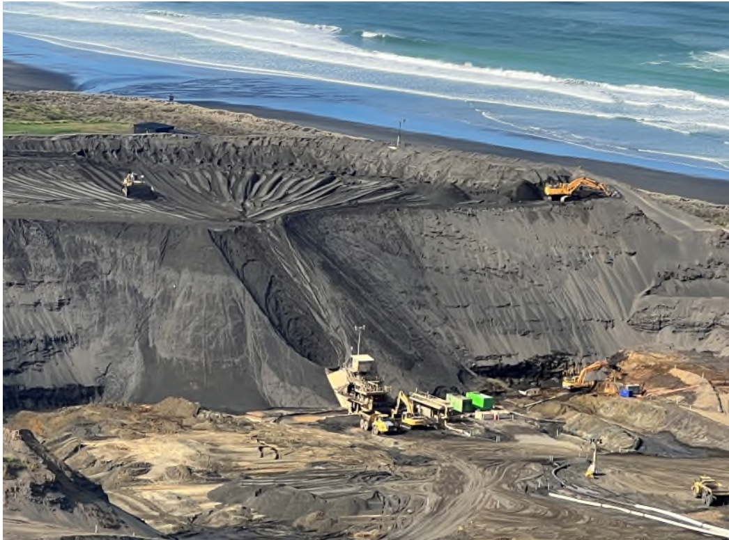
Figure 2: The mine uses dry mining methods that then form a slurry for shipment Dry mining methods at Taharoa
