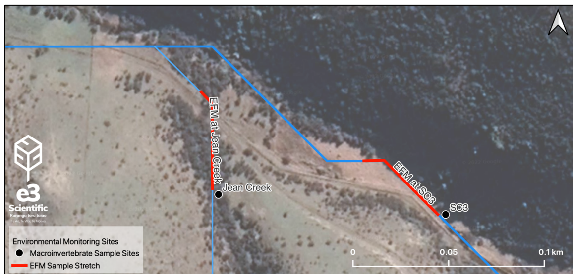
Figure 13: EFM sampling stretch example for upper Shepherds Creek (site SC3 and Jean Creek). EFM sampling was conducted for 50 m stretches downstream from the identified macroinvertebrate sample sites.
