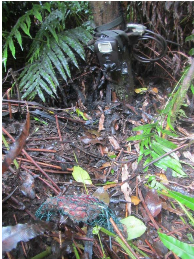
Figure 7: Camera trap set-up with the lure (comprising 150 g fresh rabbit meat between two pieces of Connovation's Erayz wrapped in chicken wire) pegged to the ground c.60cm in front of the device. Image from DOC's interim camera trapping guidelines (Department of Conservation, 2023).
