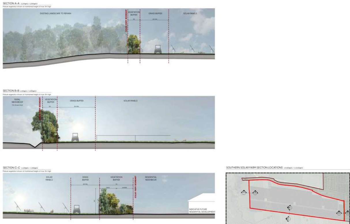
Figure 15: Indicative sections at the boundary with neighbouring properties showing the variance between 3m and 7m buffer planting 18
