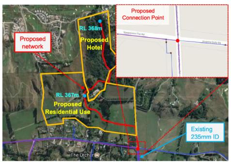
Figure 2 - Proposed Development Location, Network and Connection Point
