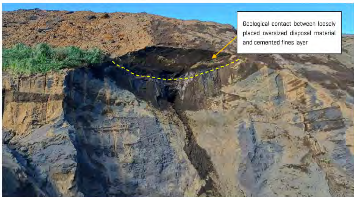
Figure 5-2 Groundwater seepage between geological contacts
