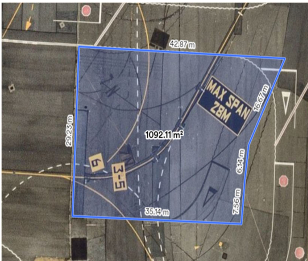
Figure 1 – Patch Repair on Taxi lane Delta R2 lead in (The MAX SPAN 28M not to be reinstated)
