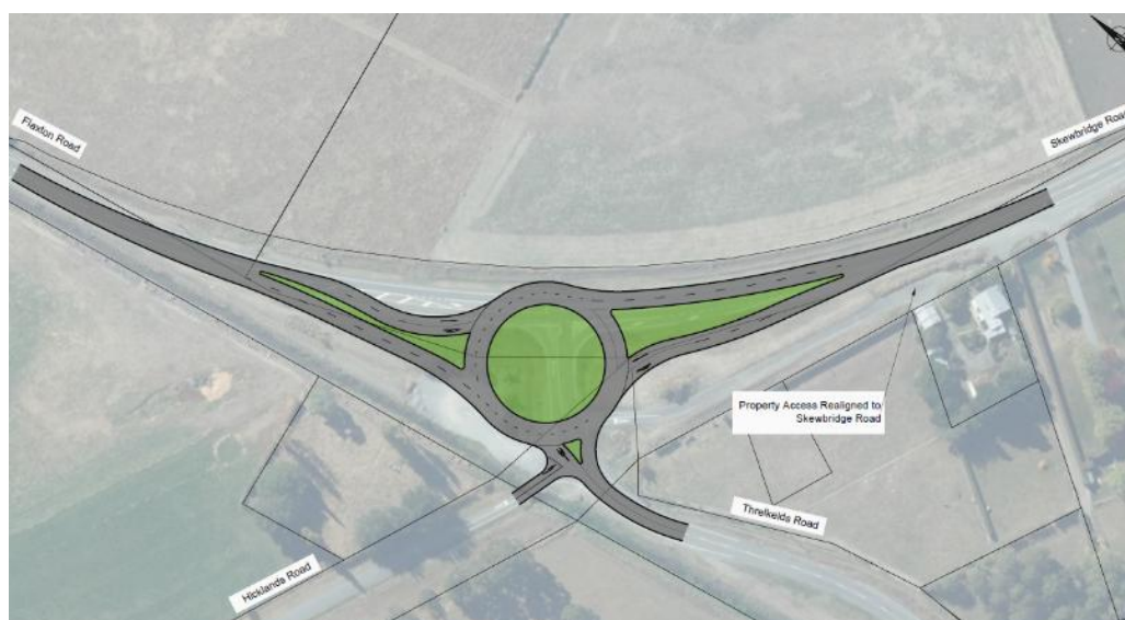
Figure 7: Recommended intersection upgrade
