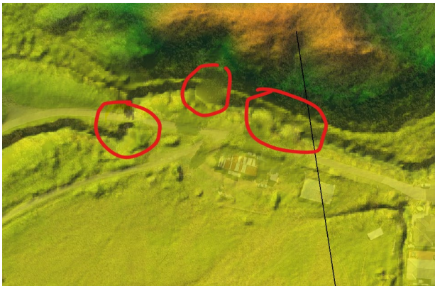
Figure 16 - Duke Road Bridge not included & DTM Issues with Stream corridor
