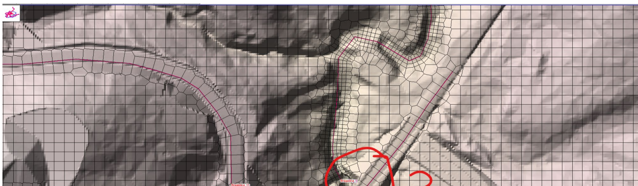
Figure 10 No culvert for the main stream channel under Forestry Road for Post Development Scenario
