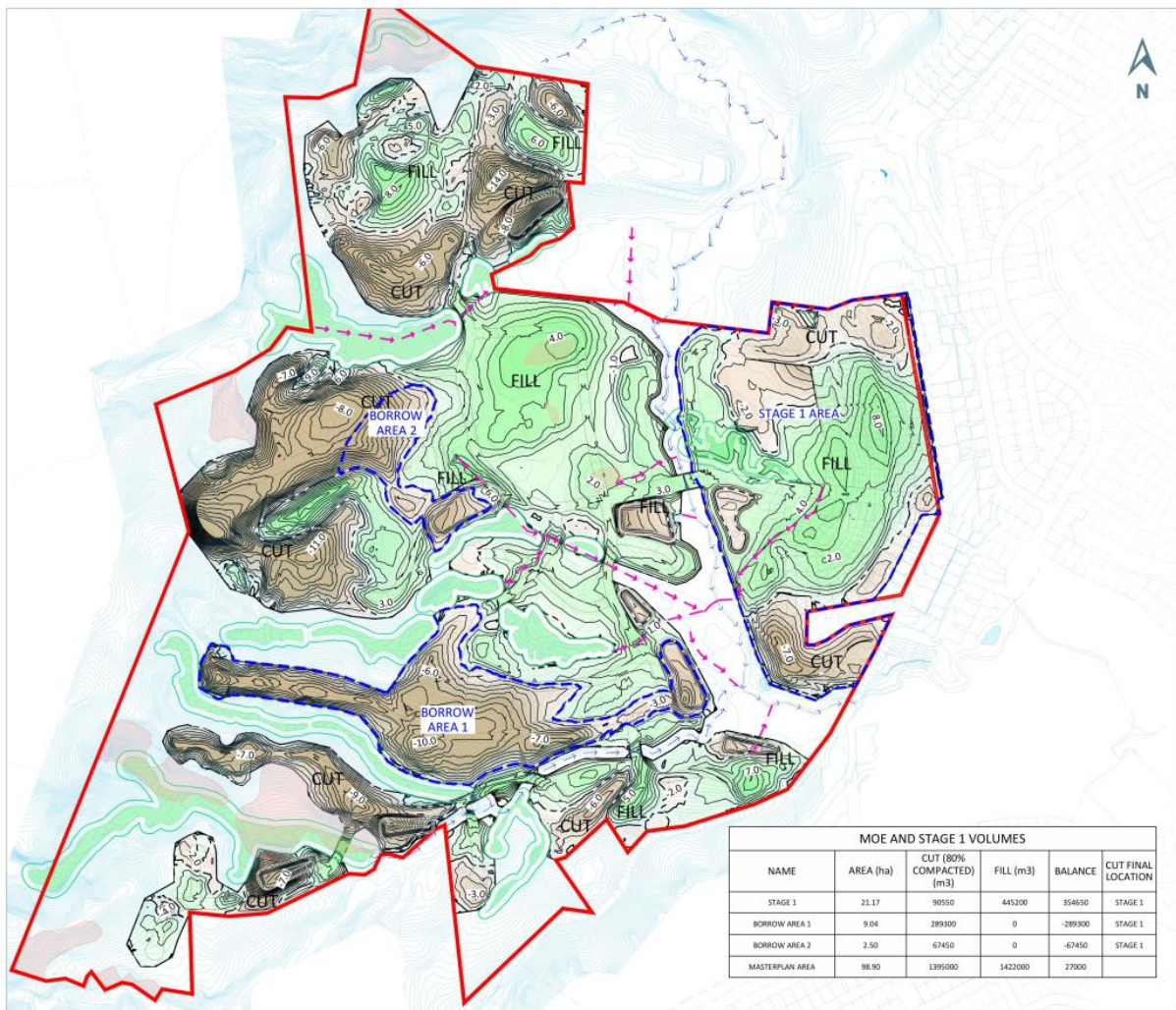
Figure 1: Pokeno West – Preliminary Earthworks
