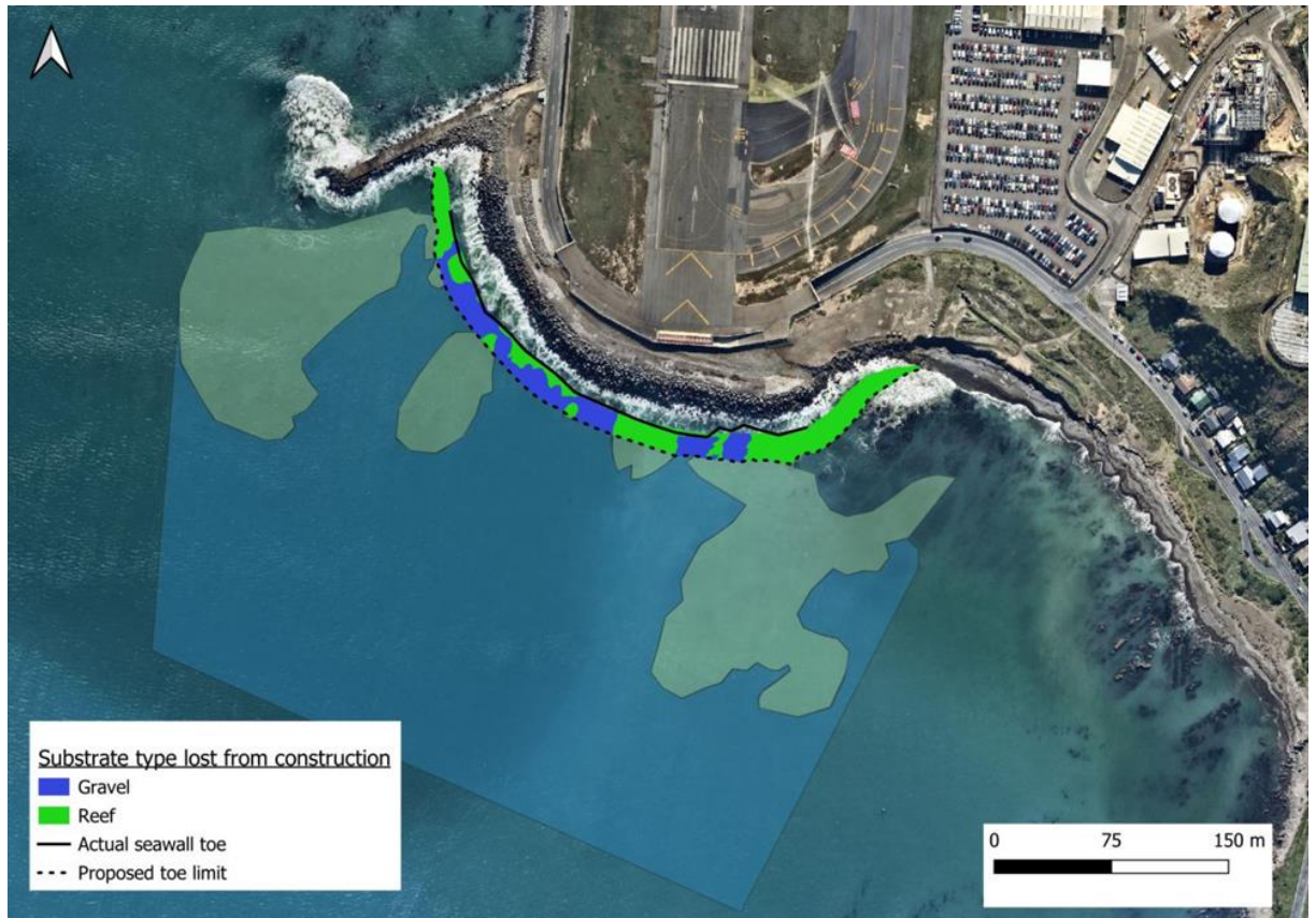
Figure 1: extent of subtidal rocky reef habitat that will be lost as a result of the placement of the seawall. Source: Figure 17 of the applicant's MEIA.
