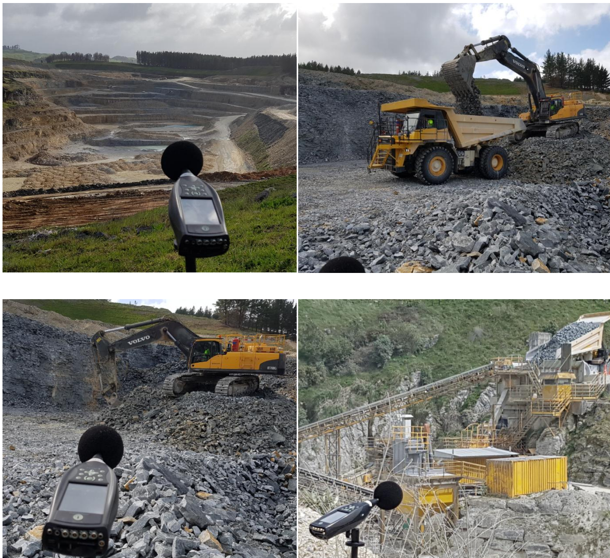
Figure 3 Examples of noise measurements performed by Styles Group at Oparure Quarry
