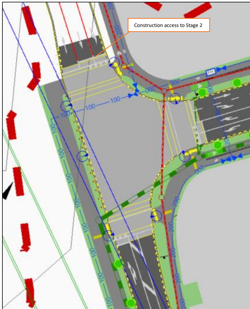
FIGURE 9: ROAD 2/ROAD 1 CONSENTED INTERSECTION DESIGN
