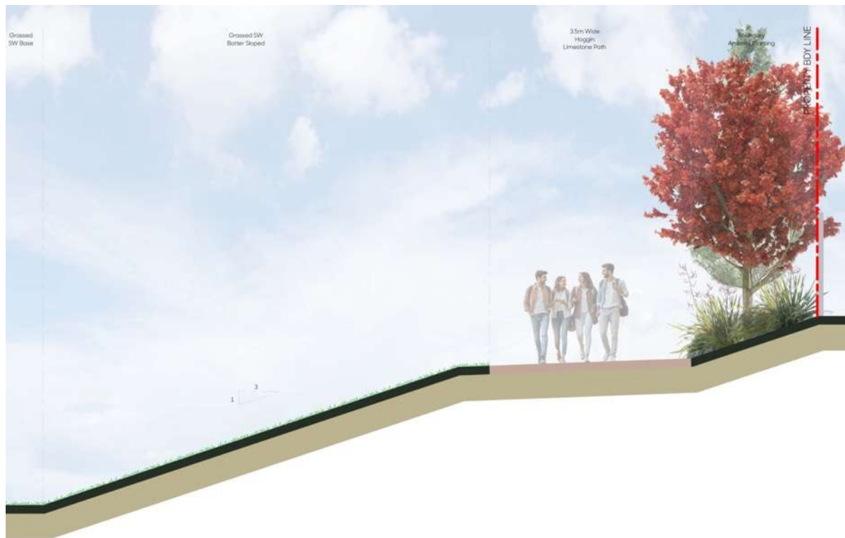
Figure 14: Typical section at Stormwater Detention basin interface with neighbouring properties 17
