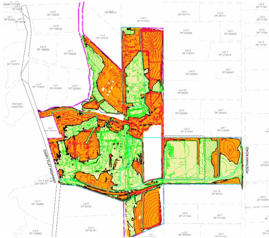
Figure 3333 – Extent of earthworks, showing cut (orange) and fill (green) (Source: MCCL drawing set 2025)
