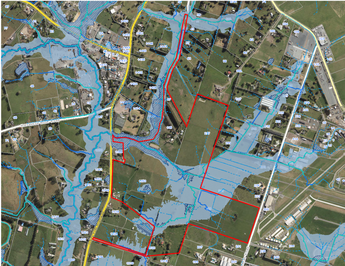
Figure 6666 – Existing OLFP (dark/light blue solid and dashed lines), Streams (cyan lines), Flood Prone Area (dashed blue area) and Floodplain (sky blue area). (Source: Geomaps, 2025)
