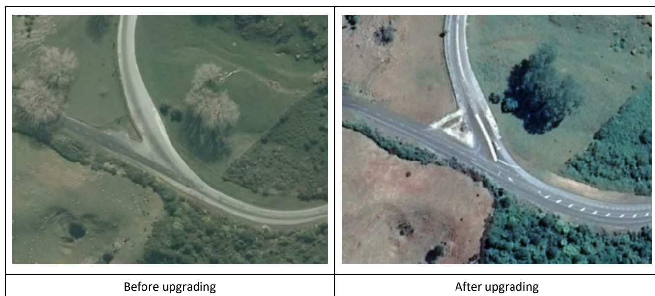
Figure 15: Quarry access changes
