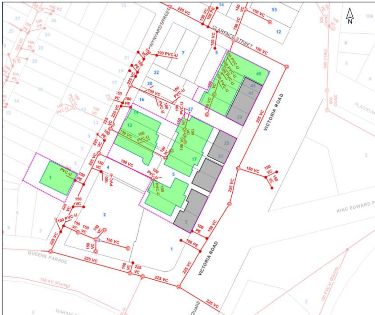
Figure 4.1: Existing wastewater services (sourced from Auckland Geomaps).
