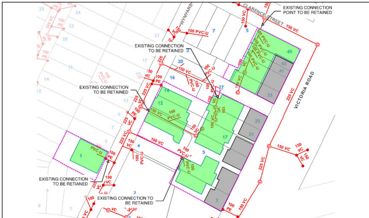
Figure 4.2 Proposed wastewater connections.
