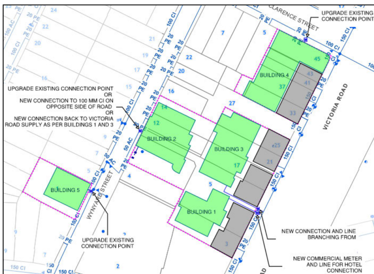
Figure 3.2 Concept water supply connections.
