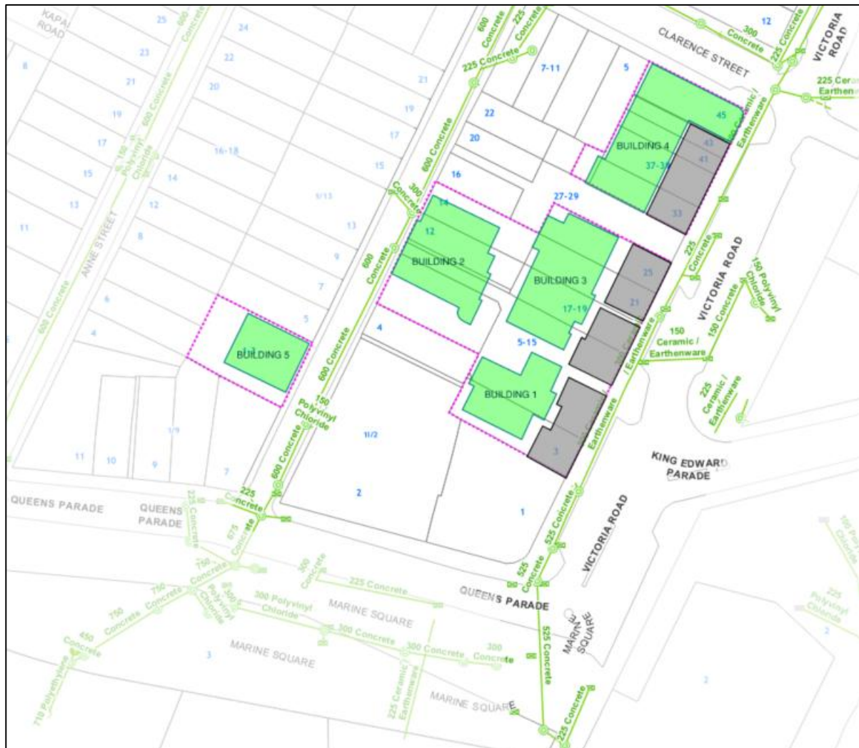
Figure 5.1 Existing stormwater services (sourced from Auckland Geomaps).
