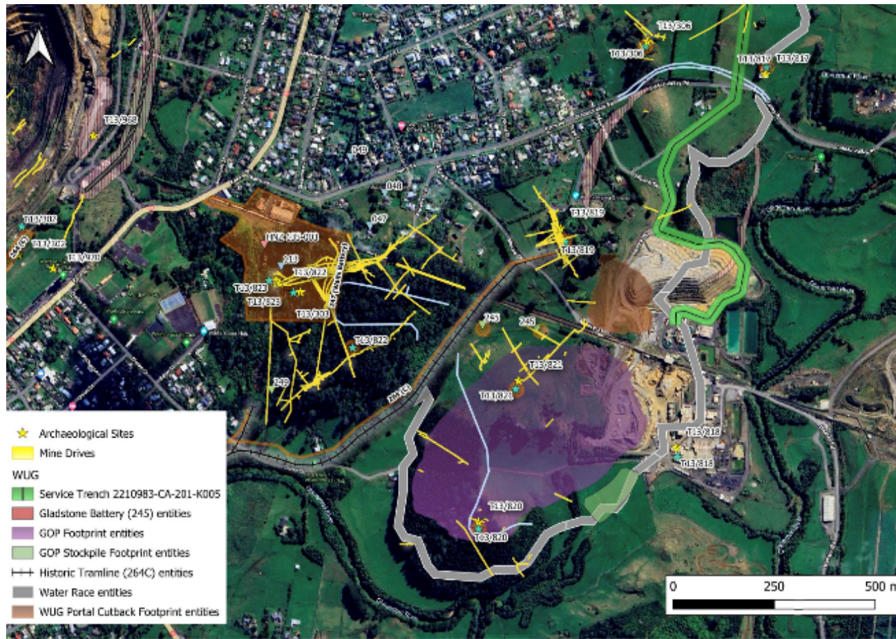
Figure 42. Recorded archaeological and other historic heritage sites within the vicinity of the Gladstone Pit (purple) and stockpile (green), WUG Portal (brown north of pit) and southern extent of the services trench (green line). The alignment of the Low Level Water Race T13/817 is shown as a grey line – sourced from NZAA ArchSite, HDP 2014 Map K4, Phillips 2000 (Features) and http://www.ohinemuri.org.nz/gis
