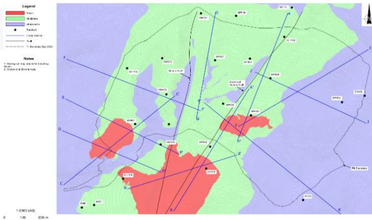
Figure 4 Geologic plan of quarry extension site, displaying distribution of geologic units at surface. Red represents distribution of volcanics, green represents distribution of WCM, and blue represents distribution of the Waipapa Greywacke which underlies the entire site. Faults can be seen in black and proposed pit extent is a black dashed line. Note that this figure displays the proposed 50-year quarry extent as provided by Terra Mining. Cross sections for geotechnical assessment are shown in blue.
