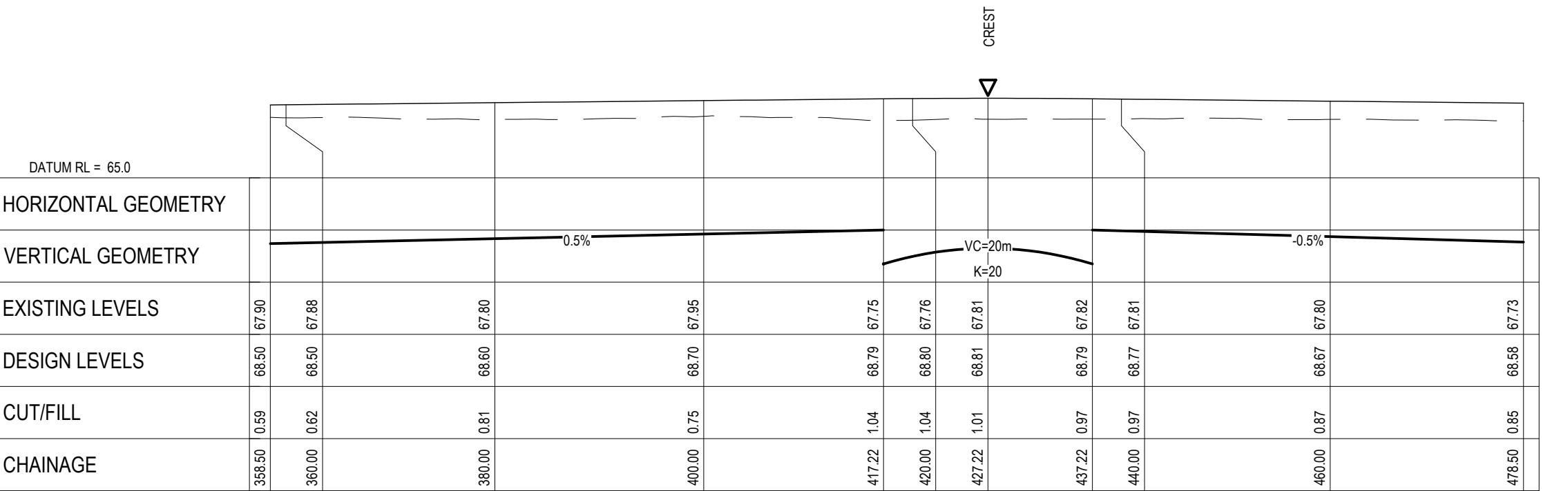
ROAD 5 LONGITUDINAL SECTION SCALE HORI 1:500 VERT 1:250
