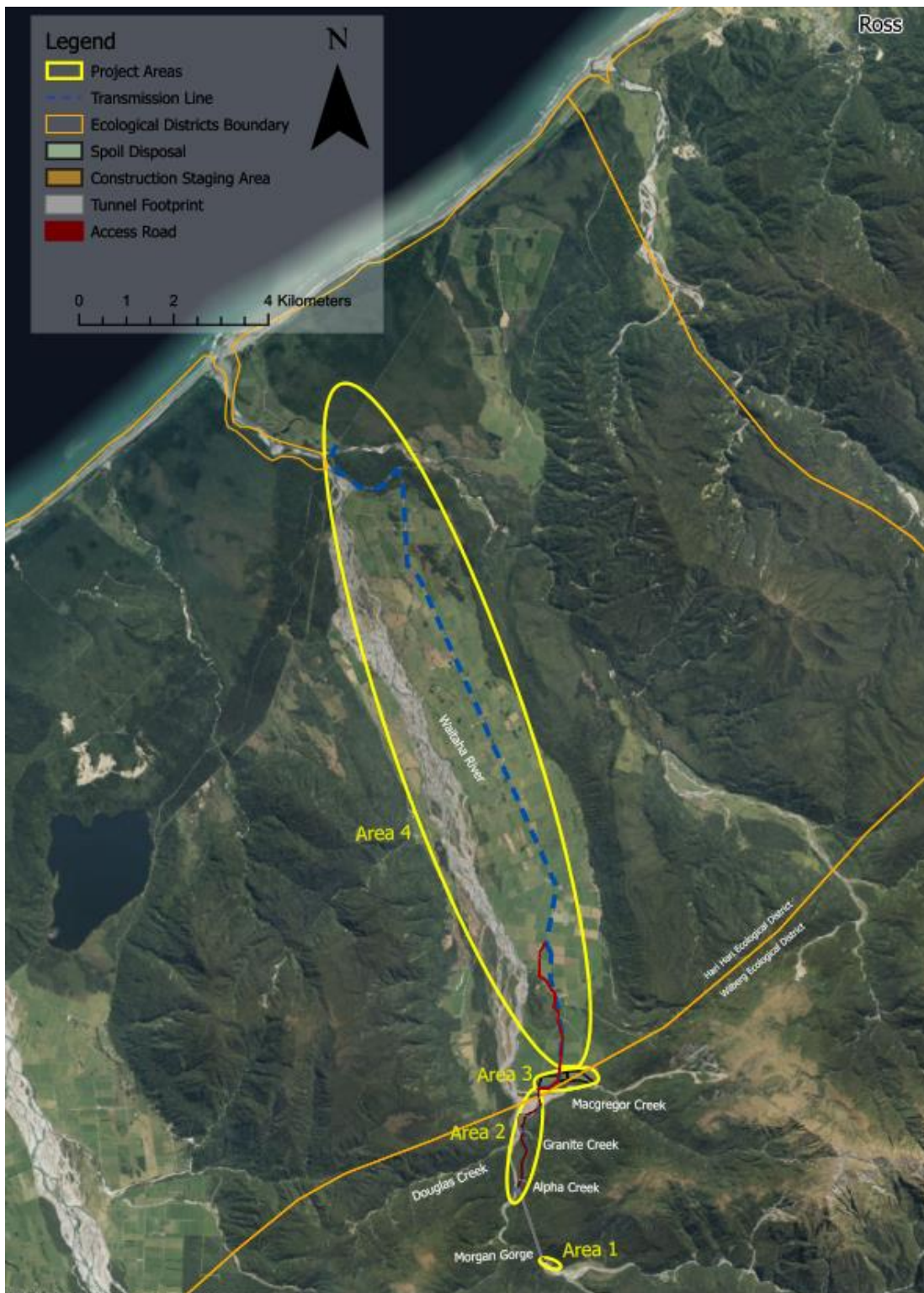
Figure 3: Waitaha Hydro Scheme overview and footprint areas. (Source: Westpower)
