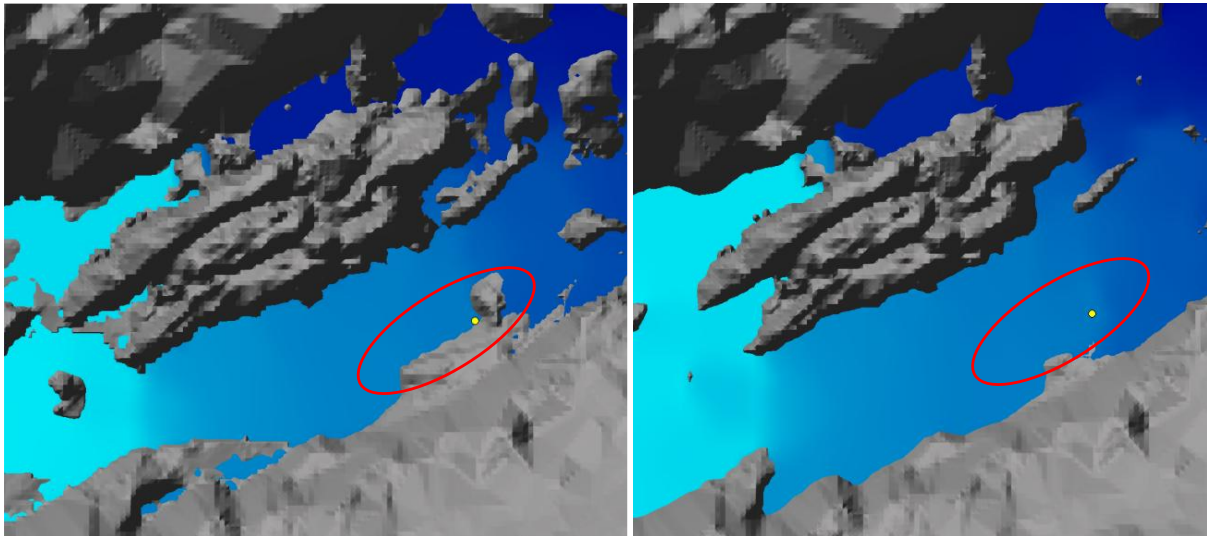
Figure 6-4: Modelled water surface at hot spring location, (left) 3.5m 3 /s, (right) 60 m 3 /s, with rock ledge indicated
