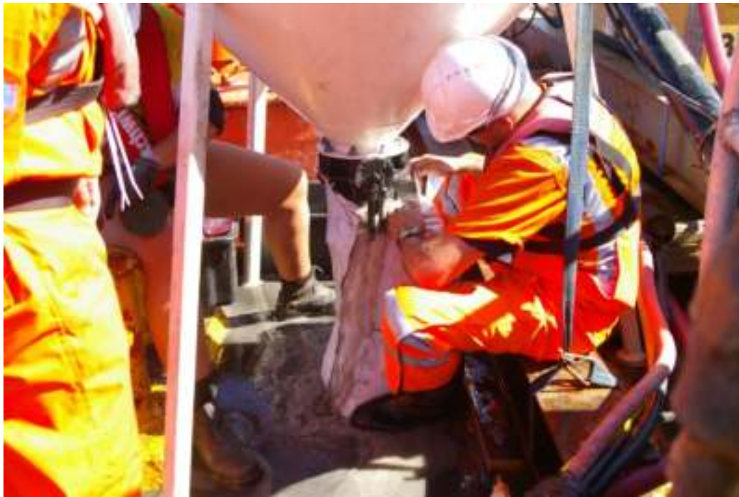
Figure 4-11 Collection of drill samples from deep drilling
