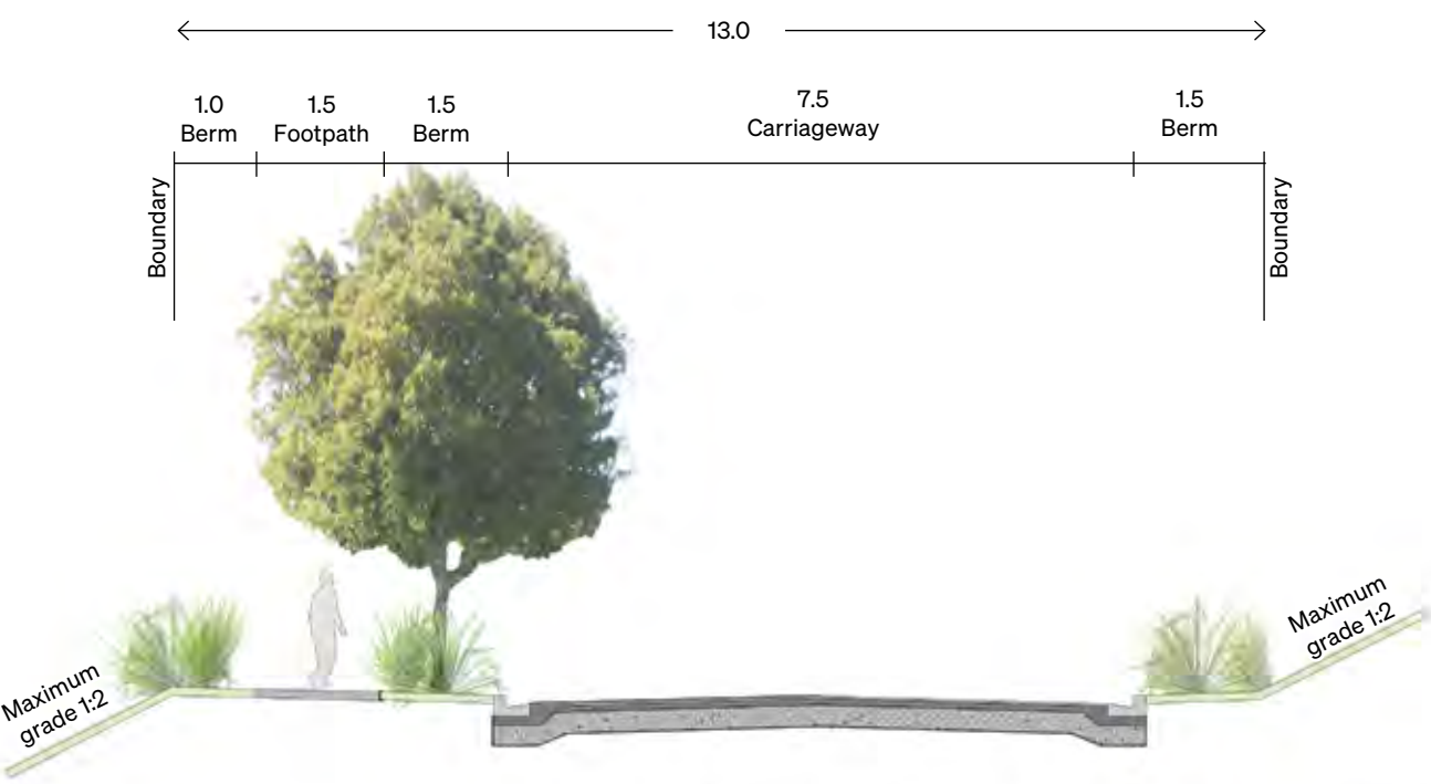
13m Interim Collector Road Planted Intersection Typical Cross Section - Roads 2 and 5. Scale 1:100 @ A3
