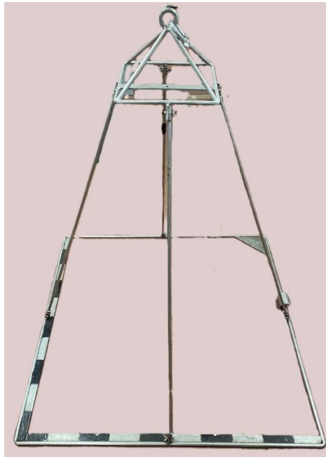
Figure 6: MBL's drop camera frame. Source: Shayne Elstob, MBL, personal communication.
