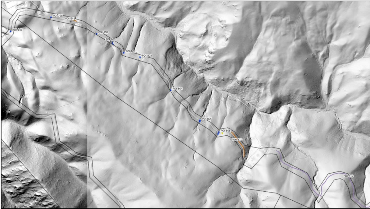
Figure 5. LiDAR imagery with land parcel boundaries shown in black. The Matakanui-Bendigo Road as surveyed is shown along with associated features. At the southeast end, the currently used road veers off to the northeast; however, a smaller narrower track continues to follow the surveyed alignment (shown in purple – POI 812), this was later determined to be a track established approximately 20 years ago, and further west it veers off from the proposed road extent. Features along the track include culverts in blue, historic drill site in yellow, and stone revetments in orange.
