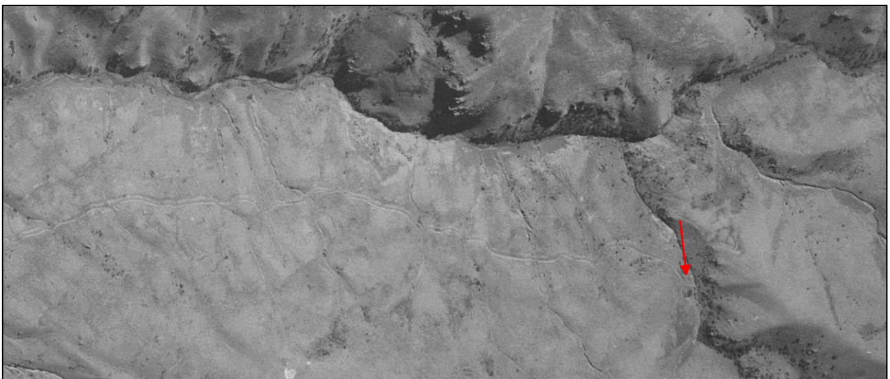
Figure 4. Aerial photograph from 1958 showing the Matakanui-Bendigo Road (Retrolens, 2021). Note that following the main stone revetment (red arrow) the wide road is no longer visible.
