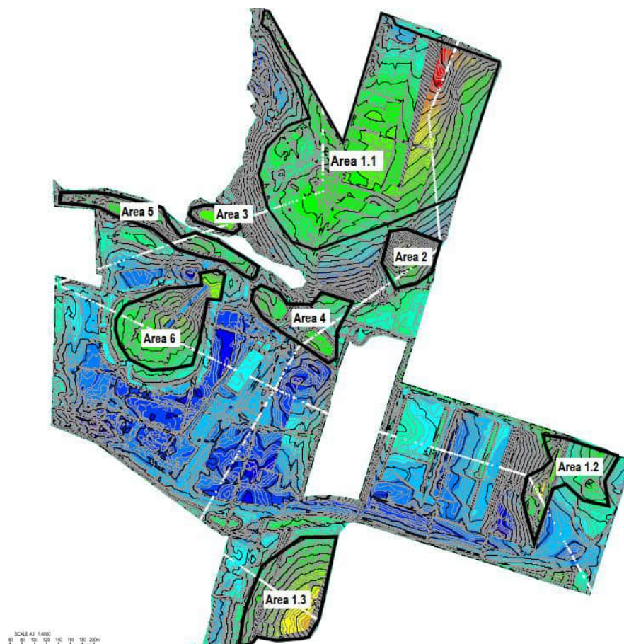
Figure 7-4: Delineation of bulk cut areas > 1m in depth. (Note: Green/yellow/red denotes net cut, turquoise/blue denotes net filling)
