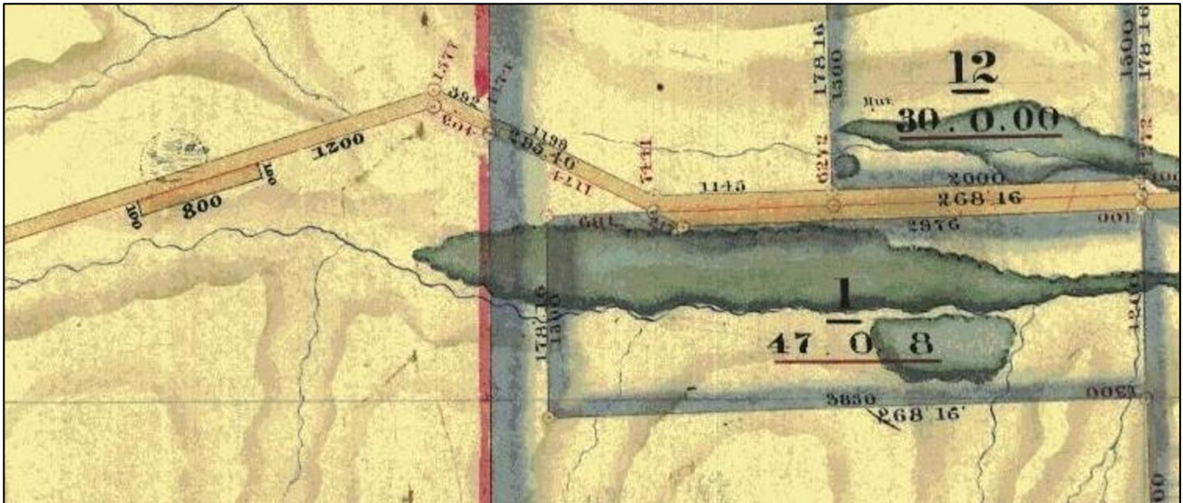
Figure 3-10 Extract of SP 736 showing Block I and II Waimumu Hundred (1869) at Bushy Park Road. Note the areas of road that are doubled in survey. Today Bushy Park Road is further south of this surveyed road and bush in the project area.
