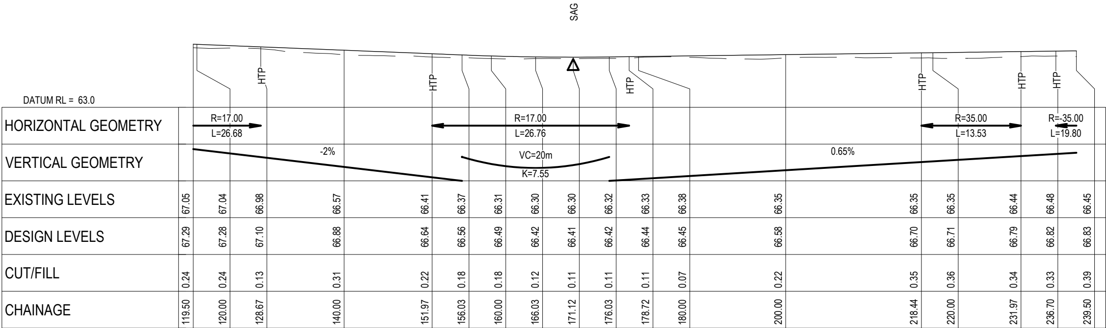
ROAD 6 LONGITUDINAL SECTION SCALE HORI 1:500 VERT 1:250
