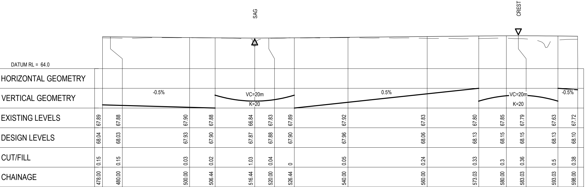
ROAD 5 LONGITUDINAL SECTION SCALE HORI 1:500 VERT 1:250
