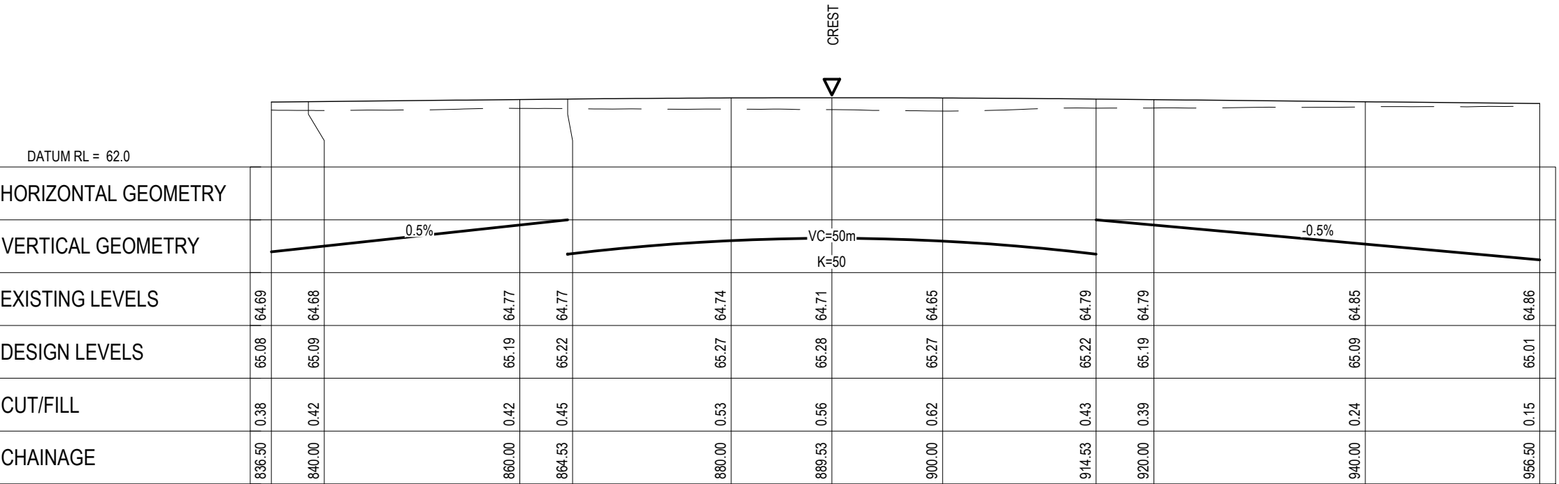
ROAD 1 LONGITUDINAL SECTION SCALE HORI 1:500 VERT 1:250
