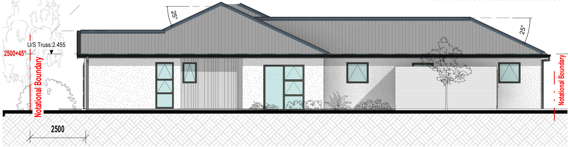
East Elevation Scale 1 : 100
