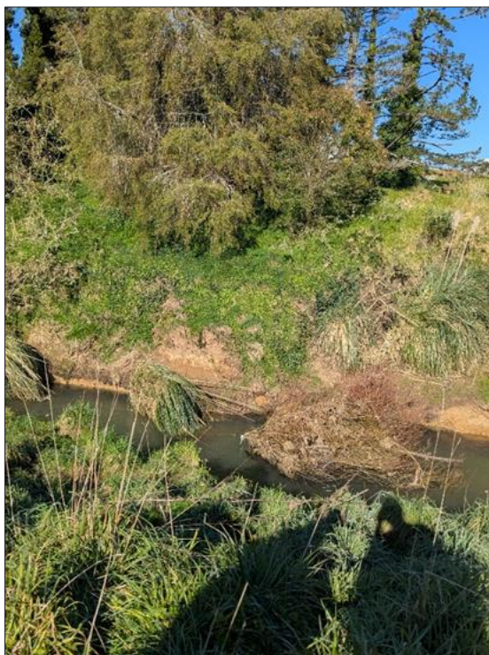
Figure A1.8: Noted debris lines and bent vegetation denoting peak flow
