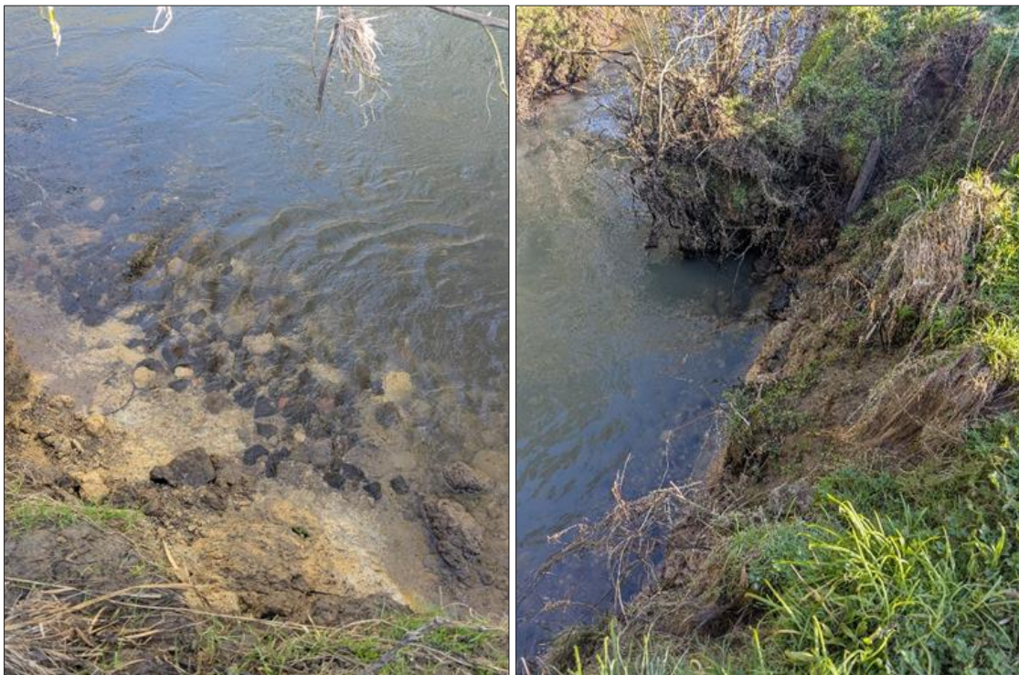
Figure A1.5: Observed mixed coarse bedload sediment
