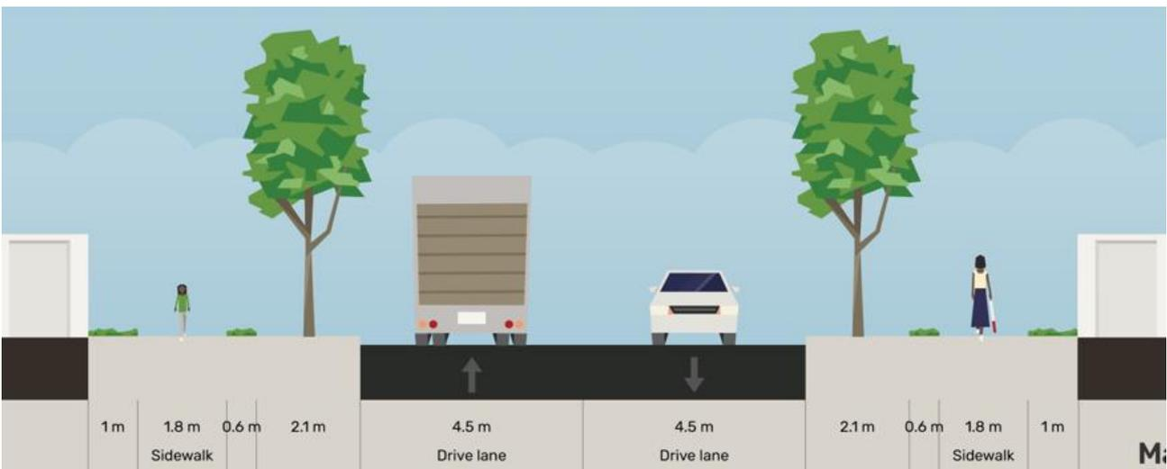
Figure 13: Typical Cross-Section – Industrial Local Road
