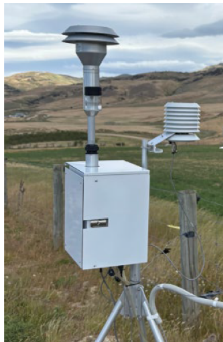
Figure 5: Photograph of real time dust monitoring equipment
