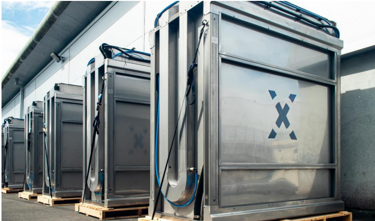
Figure 6: Example of OxyMem type MABR modules prior to installation inside tank. Each module houses gas permeable membranes which provide a growth surface for the biomass.
