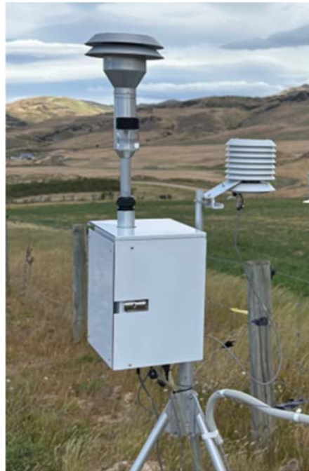
Figure 885: Photograph of real time dust monitoring equipment
