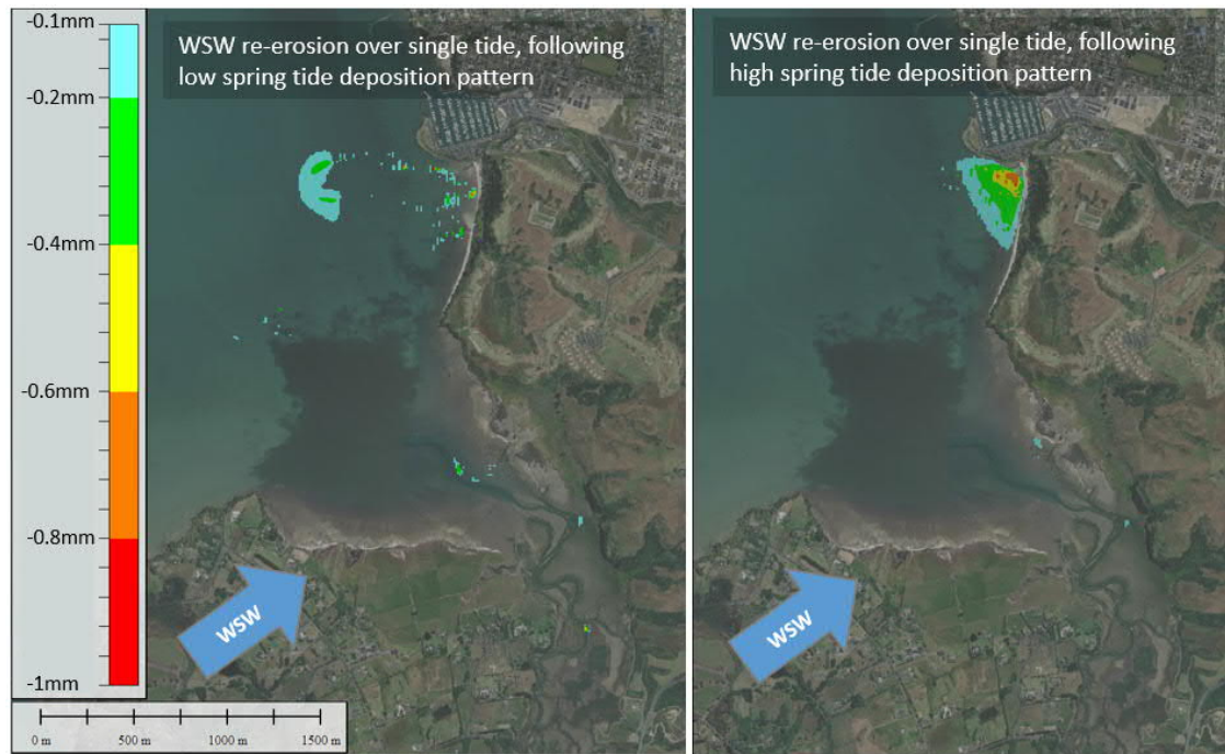
Figure 4-7 Comparing re-erosion rates of lower (low tide) and upper (spring tide) deposition areas
