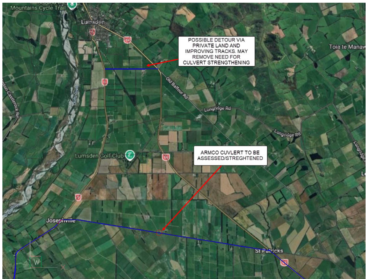
1-7 Culvert strengthening or bypass on Josephville St Patrick road
