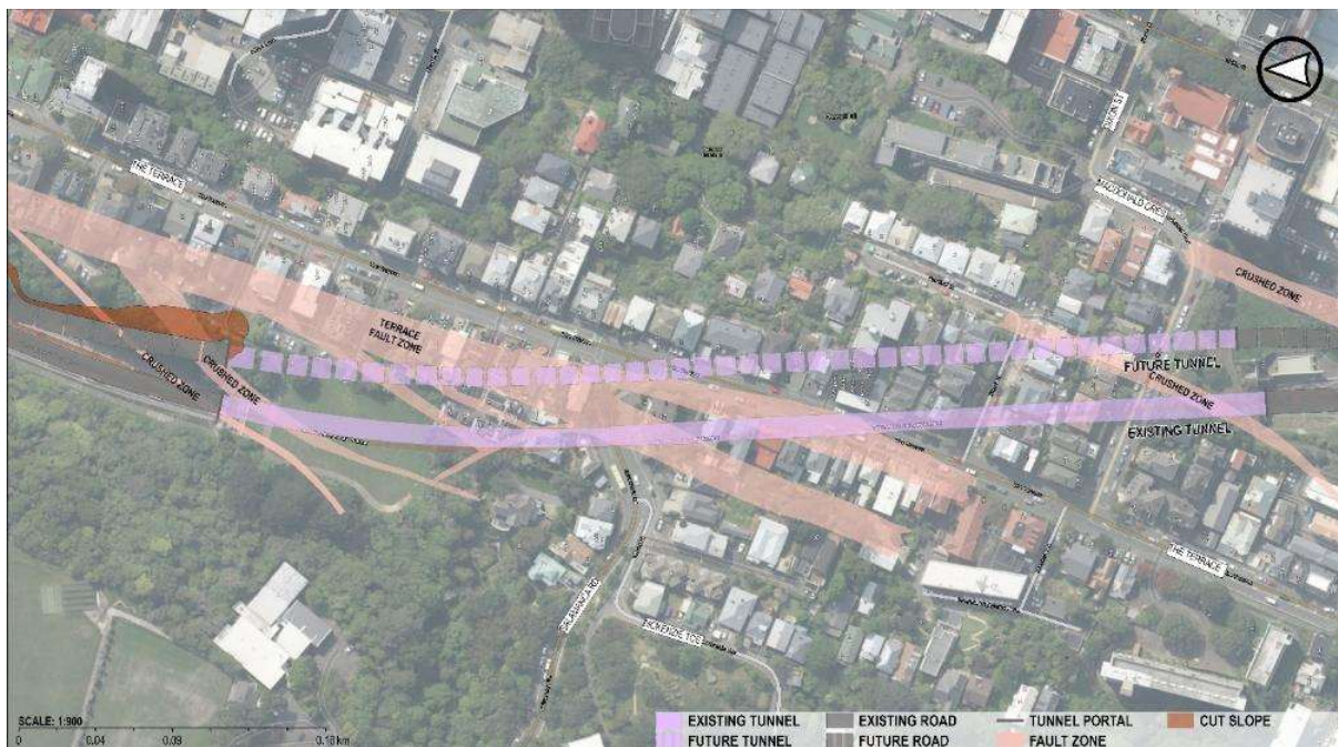
Figure 44 – Terrace fault zone along the proposed northern approaches to the southbound tunnel (after Beca, 2015)
