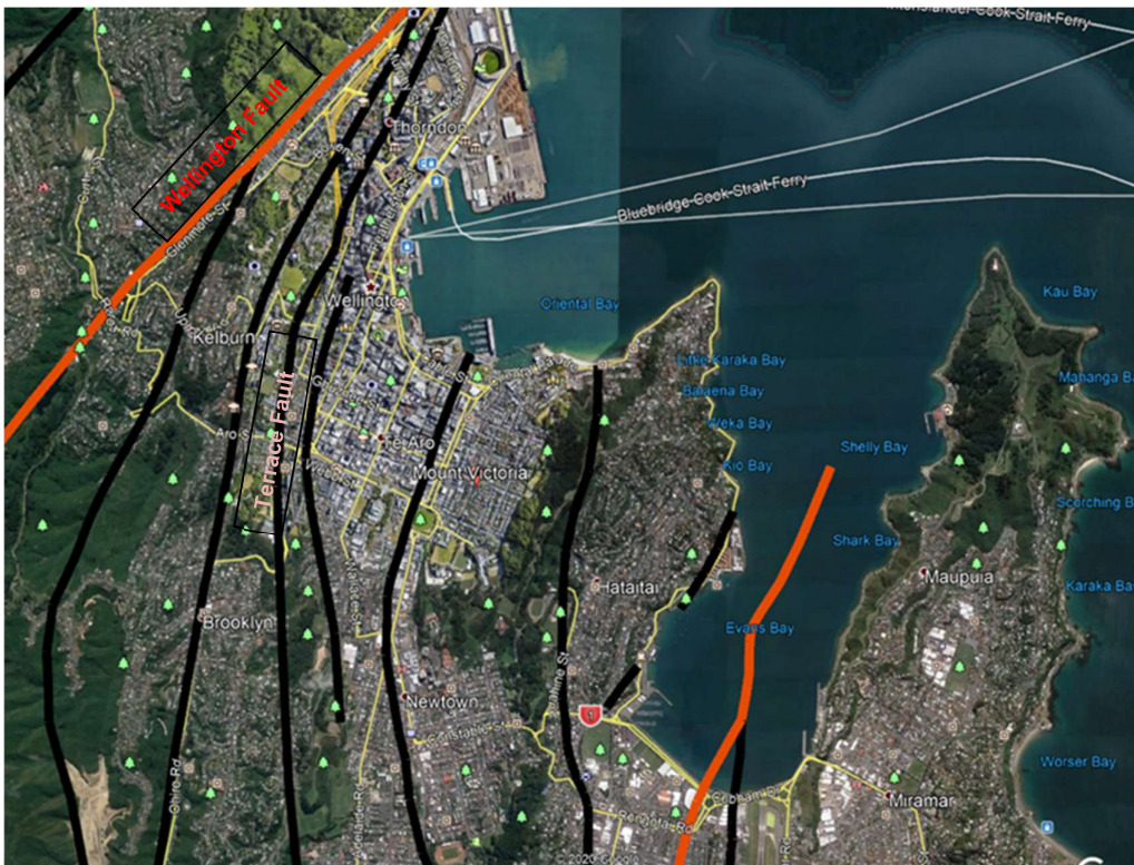
Figure 4 – Active and other faults in the Wellington CBD and eastern suburbs (after GNS, 2000)
