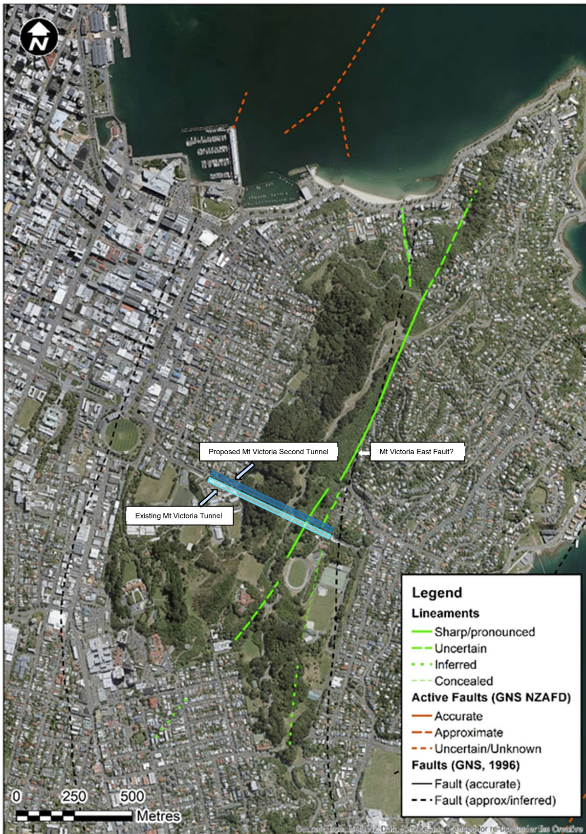
Figure 7 – Location of Fault, east of Mt Victoria (black), and lineaments from LiDAR
