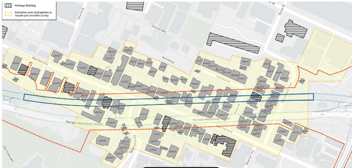
Figure 38 – Area of potential subsidence and heritage buildings near the proposed second tunnel
