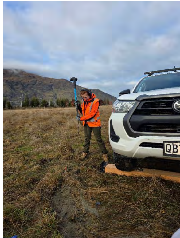
Figure A2: Striking the shear wave source.
