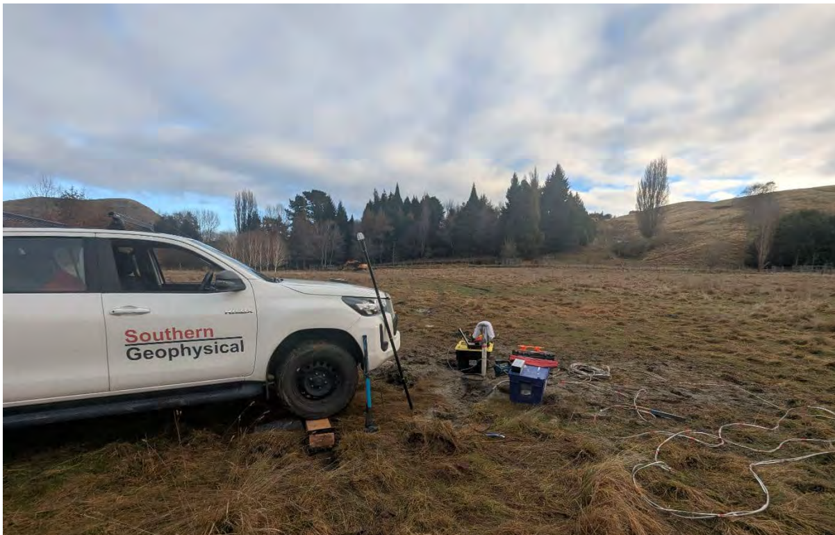
Figure A3: Shear wave source weighted down by the truck and equipment set up.
