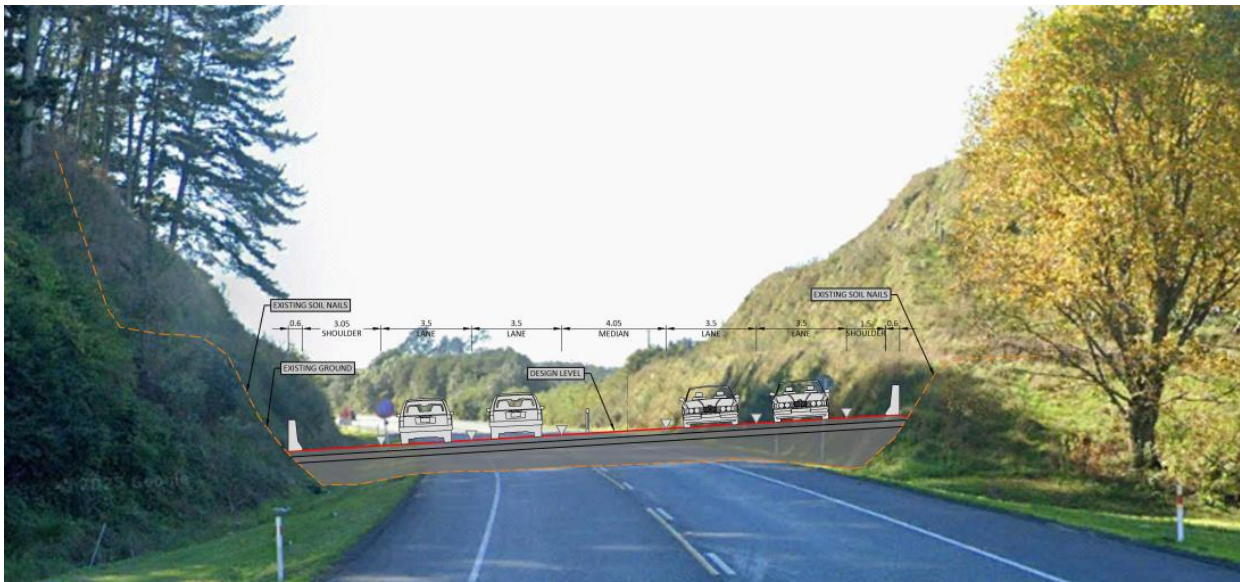
Figure 9: Example of the carriageway profile adjacent to the Puketoromiro pā
