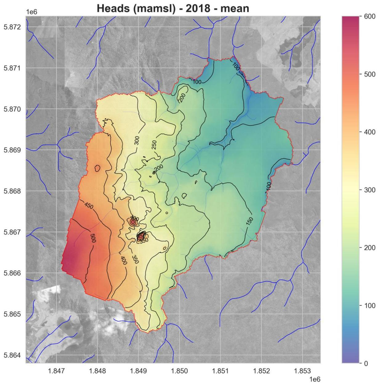
Figure 4-5 - Simulated mean steady state (pre-mine) water table.
