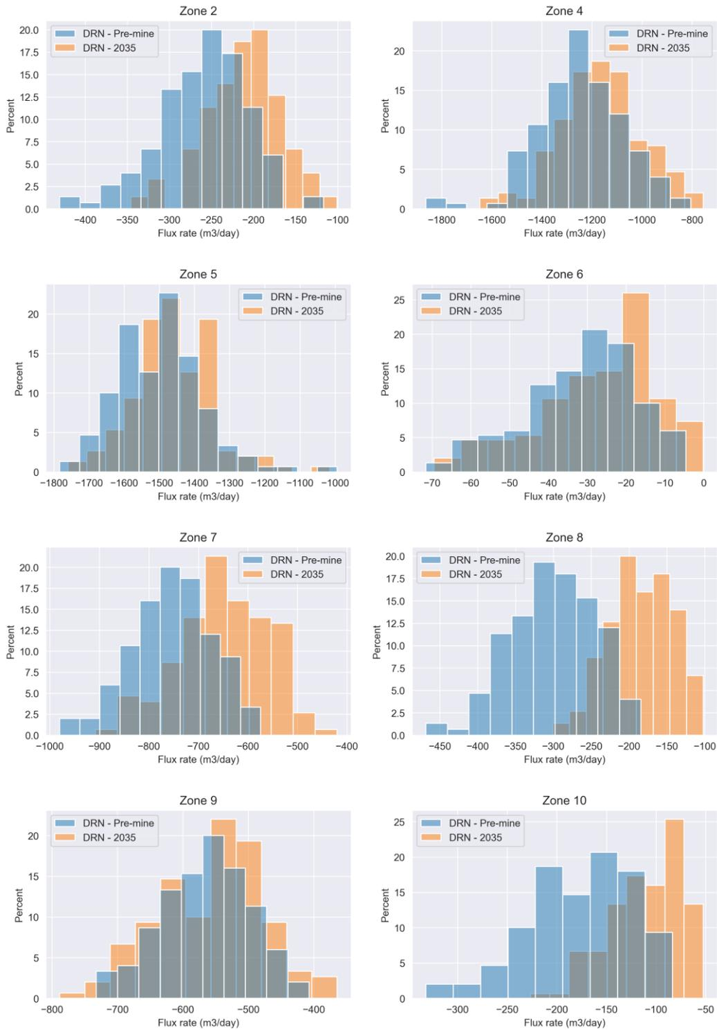
Figure 4-3 – Simulated drain boundary water fluxes pre- and post-mining<sup>2</sup>.
