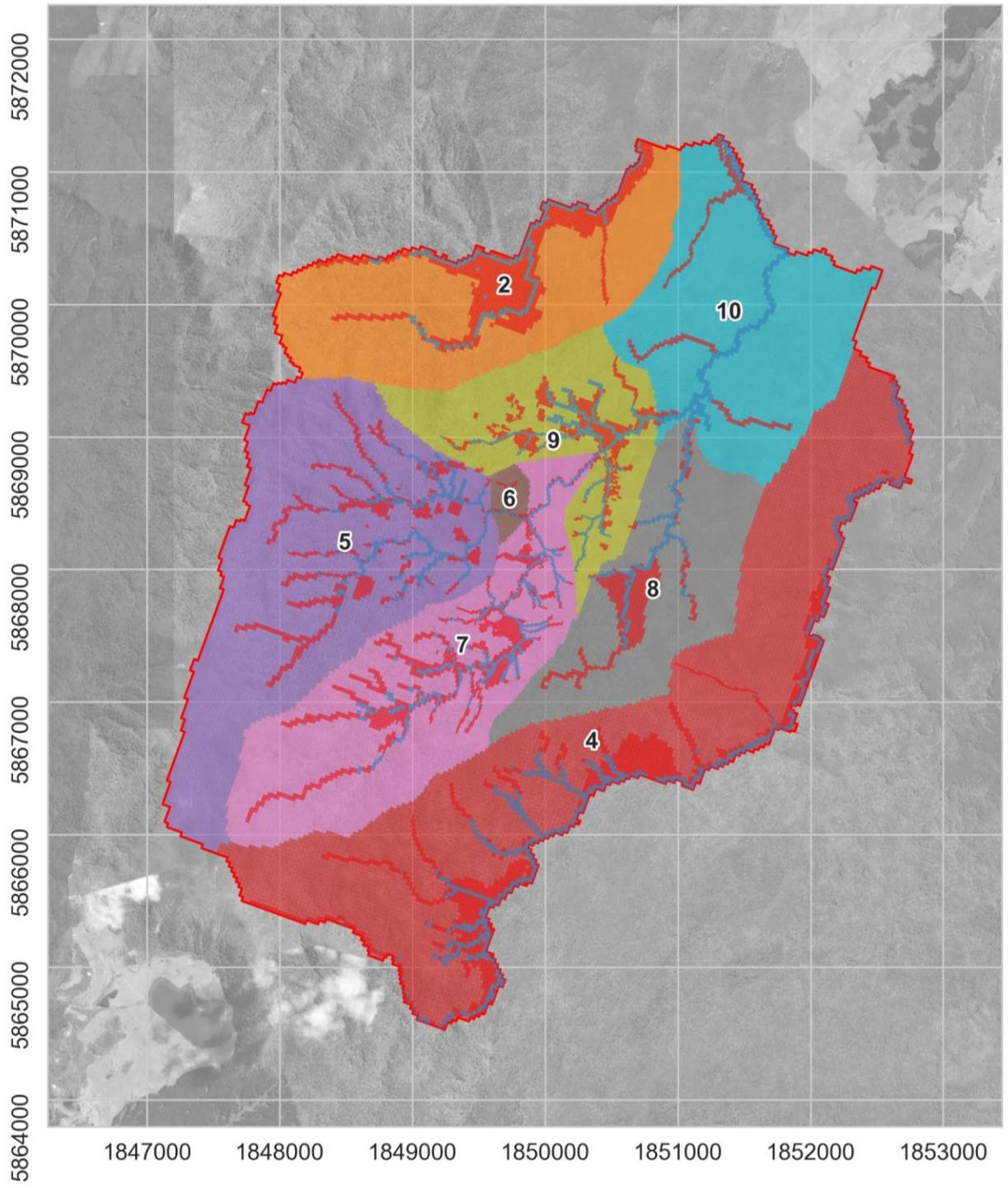
Figure 4-1 - Surface water zones and boundary conditions (red cells – drain boundaries, blue cells – river boundaries).
