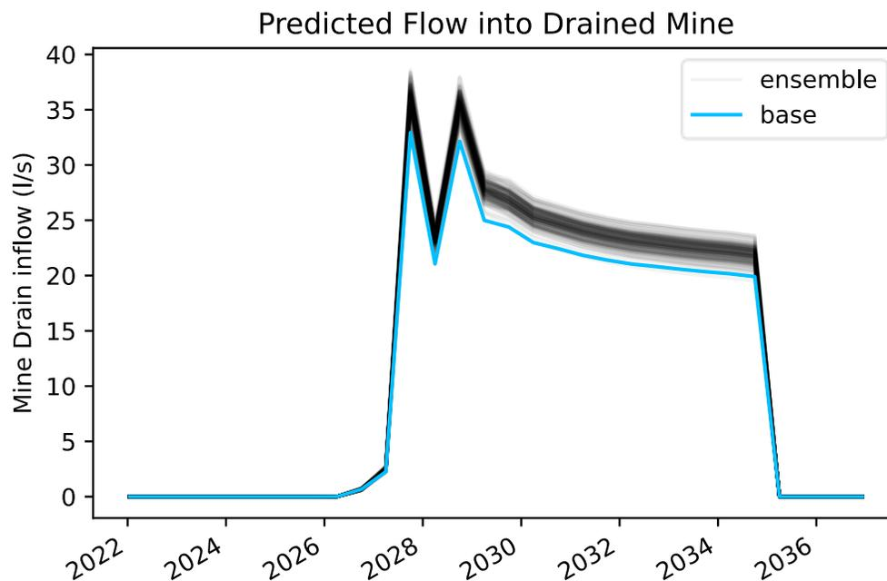
Figure 4-4 - Predicted flux rates into the mine.
