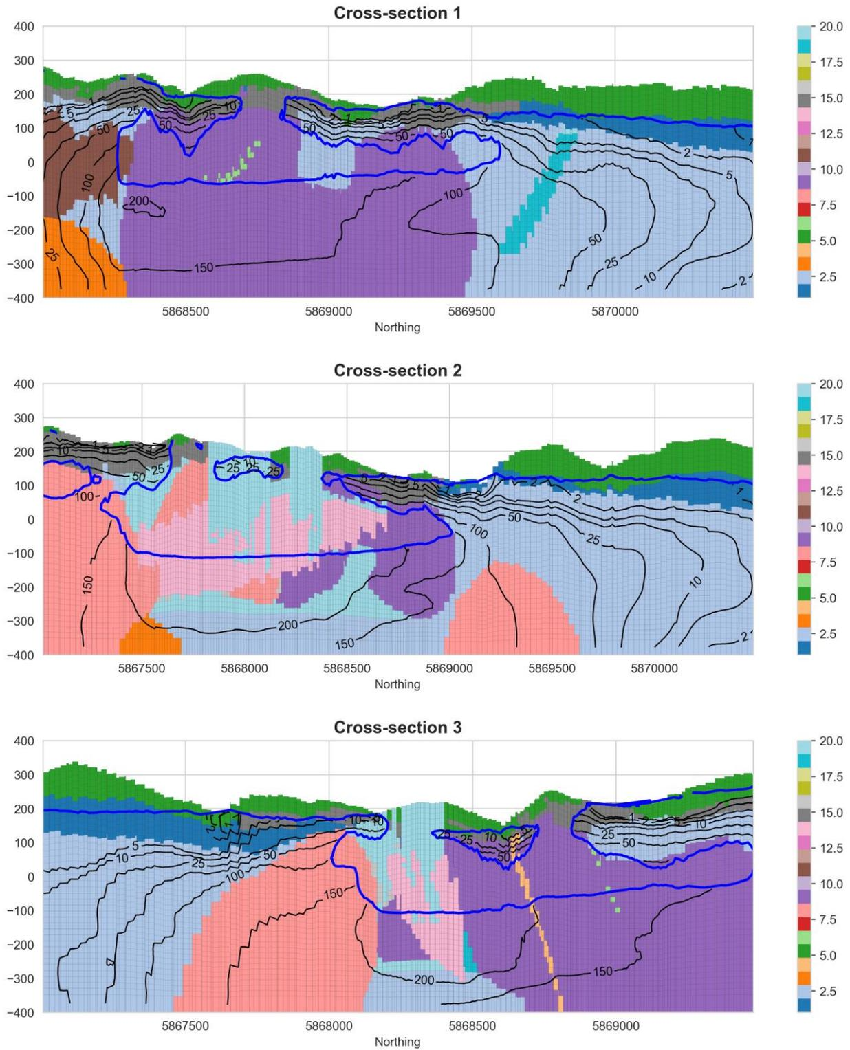
Figure 4-11 - Simulated mean 2035 (end of mine) drawdown contours (black) and zero-pressure isoline (blue), shaded by HSU code.
