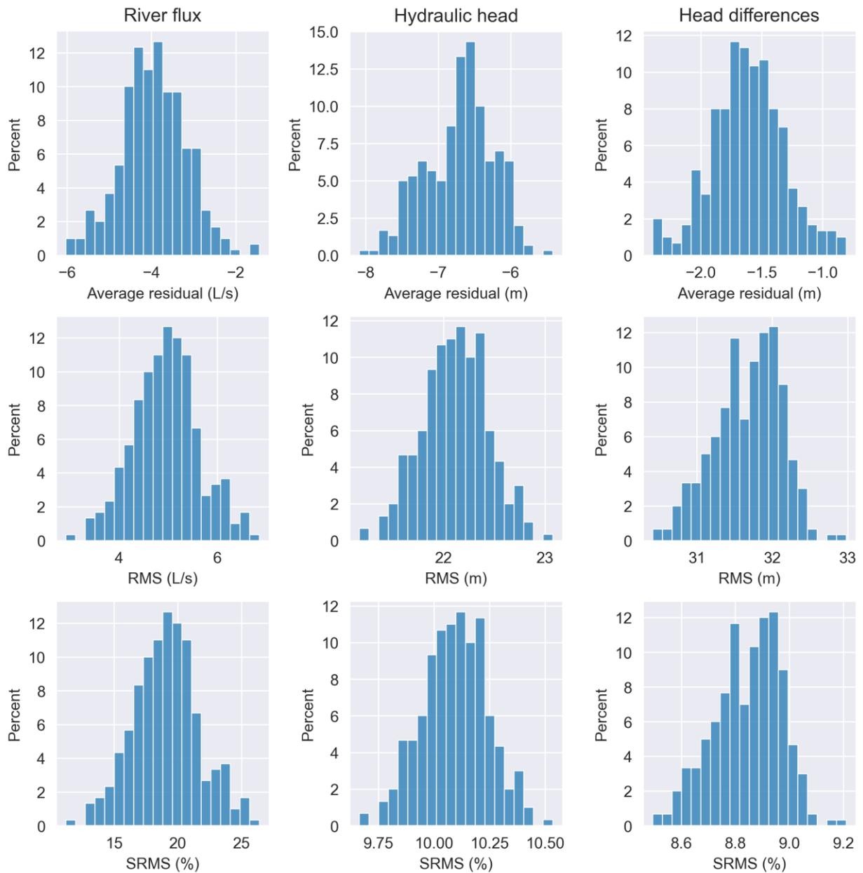
Figure 3-4 – Calibration histograms for all realizations, grouped by observation type and calibration metric.
