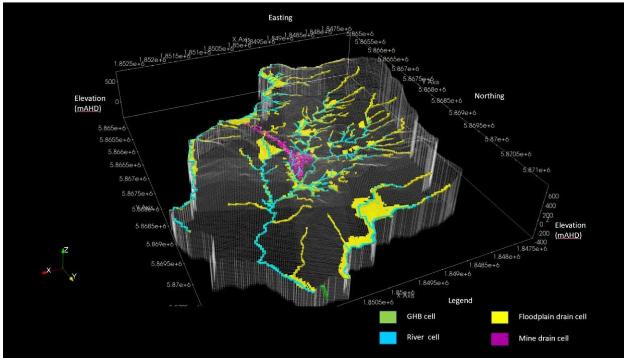
Figure 1-3 - Boundary conditions of predictive model showing drain cells (yellow), river boundaries (blue), general head boundary cells (green) and drain cells representing mining at WUG (pink).
