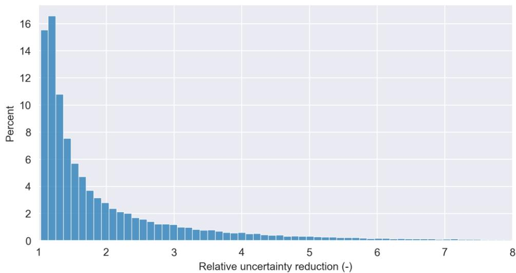
Figure 3-6 - Histogram of parameter uncertainty reductions (pre- / post-calibration standard deviations) for all parameters.
