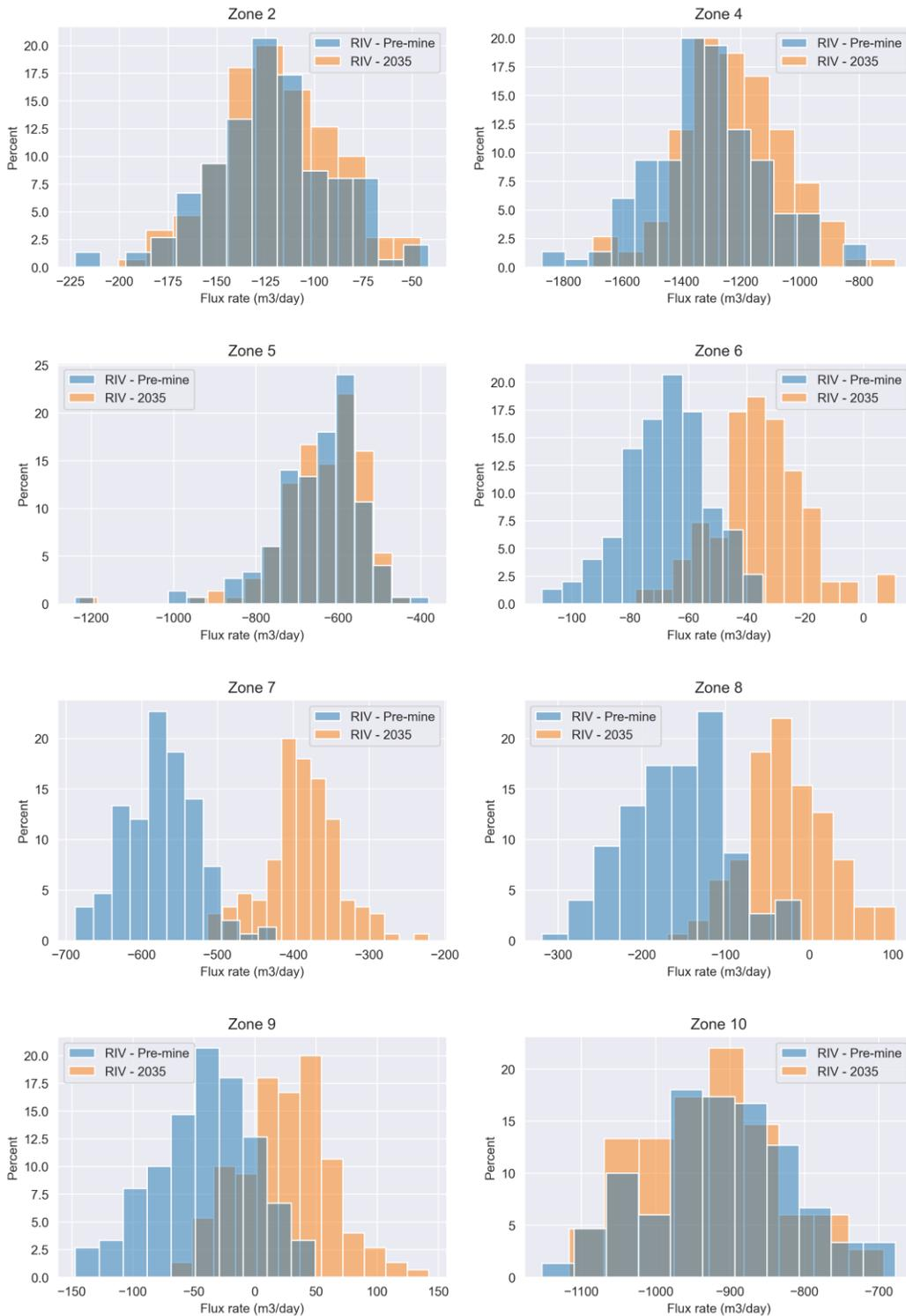
Figure 4-2 – Simulated river boundary water fluxes pre- and post-mining<sup>1</sup>.
