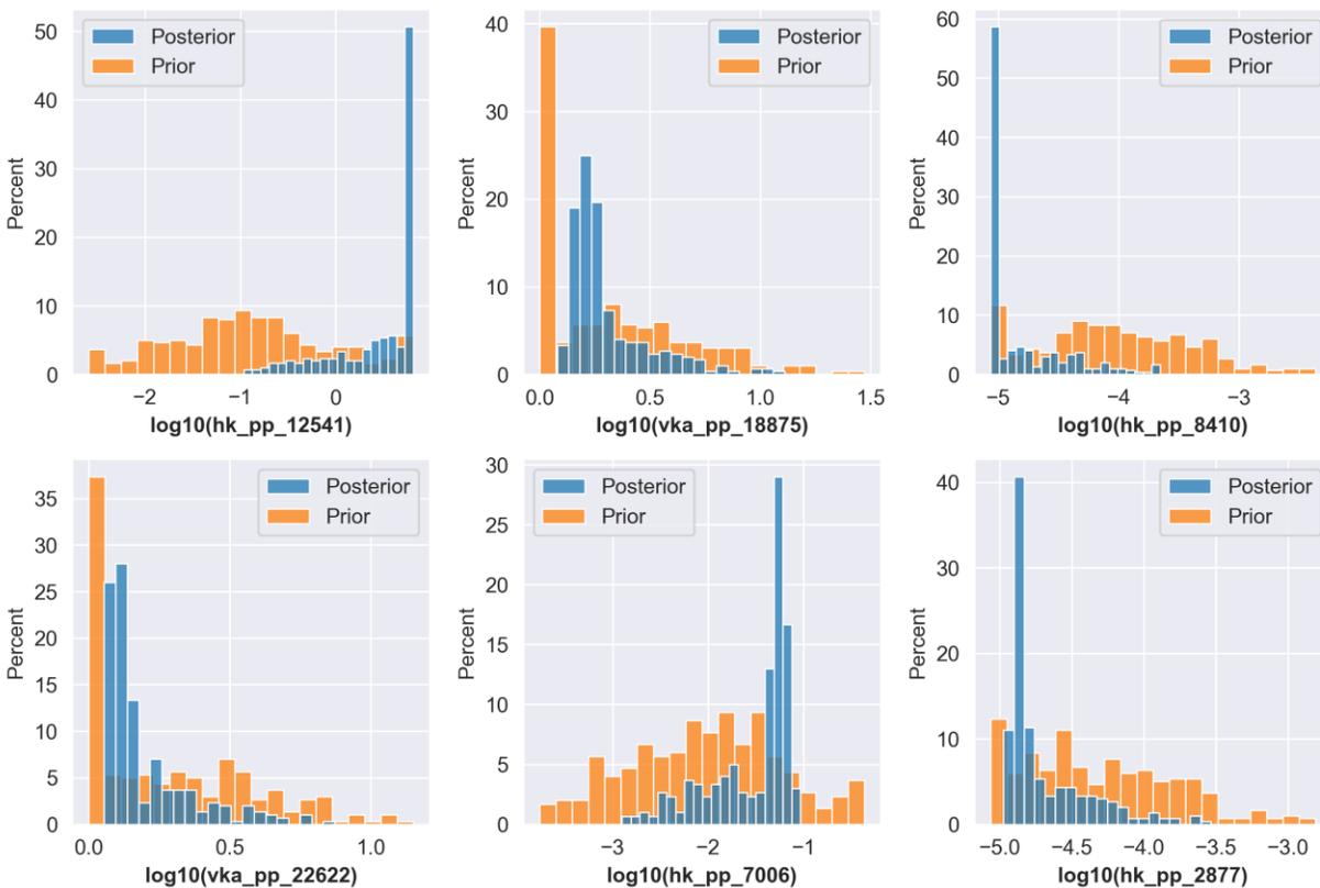
Figure 3-7 - Comparison of pre- and post- calibration values for selected parameters (hk – horizontal hydraulic conductivity in m/d, vka – vertical anisotropy Kh/Kv).
