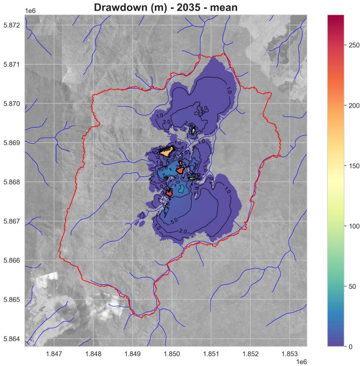
Figure 4-6 - Simulated mean 2035 (end of mining) drawdown.
