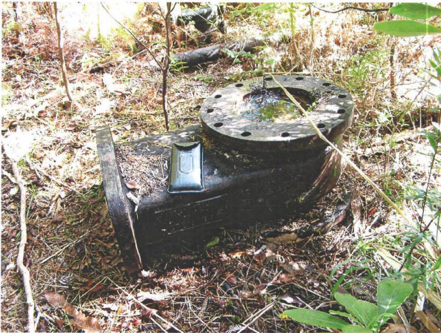
Figure 10 Hydraulic joint, battery site WP 299. Inscription on side reads: "Glenfield and Kennedy Ltd Kilmarnock".
