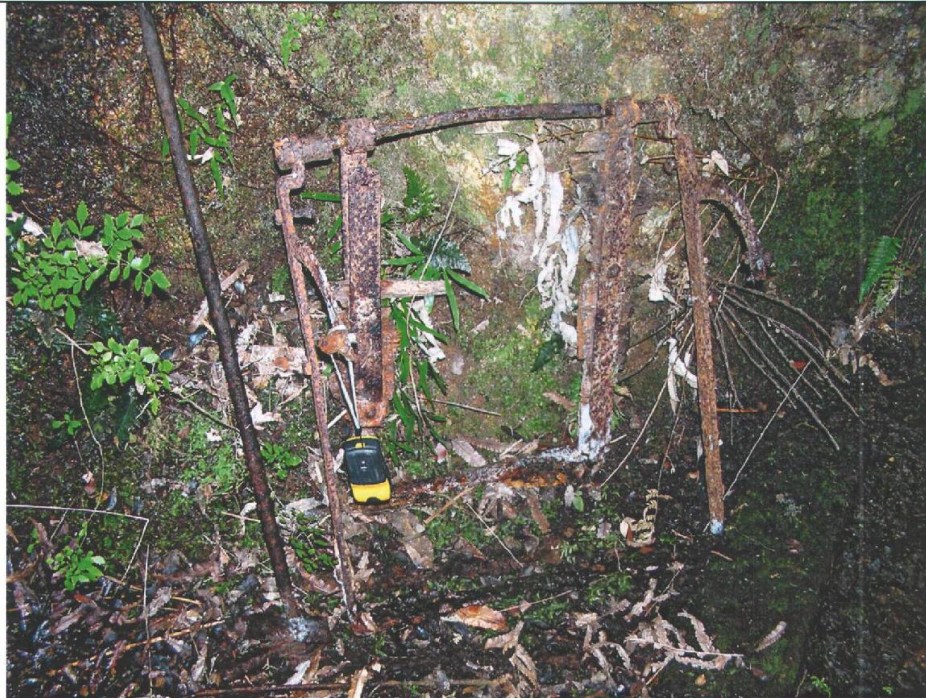
Figure 19 Metal remnants in adit entrance WP 314 (probably the tipping mechanism for a cart)
