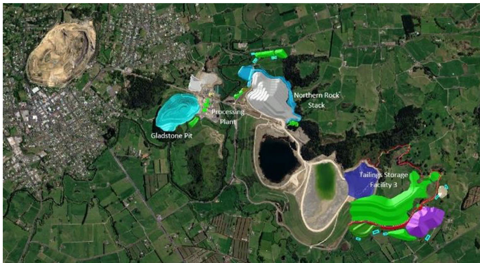
Figure 2. WNP proposed expanded Waihi operations – Gladstone Open Pit (GOP), Processing Plant, Northern Rock Stack (NRS) and TSF3 Storage Facility ((source: Oceana Gold)
