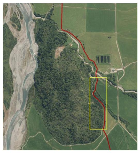
**Figure 6.** The Doughboy (forested hill) with proposed main access road shown in red, which follows an existing farm road. The upgrade of the road from a 4 m farm track to 8 m wide access track along its current alignment (red line) will involve works within a portion of the eastern side of the Doughboy (generally, the yellow box) and this may require some limited woody vegetation clearance, as well as clearance along the existing rank grass shoulder.
