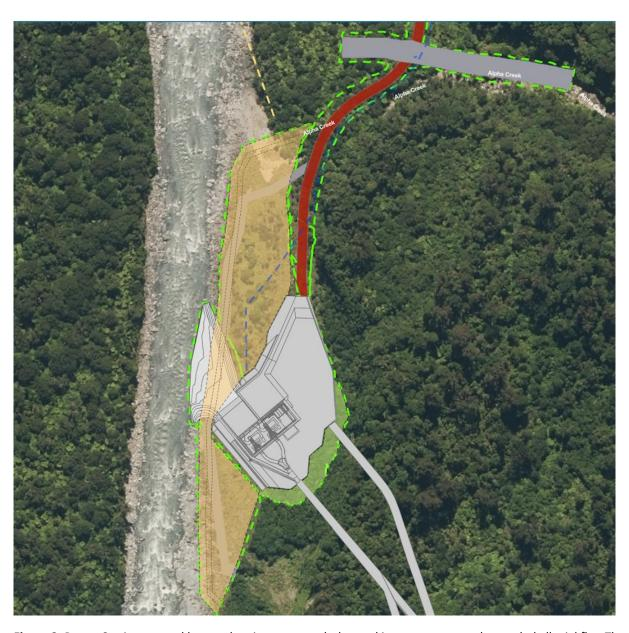
**Figure 3.** Power Station general layout showing most works located in an open, sparsely wooded alluvial flat. The transmission line and access road corridor (as shown at the top of the figure at Alpha Creek) is within the start of regenerating kamahi forest.
