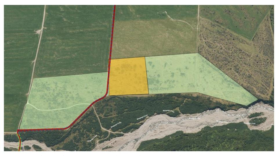
**Figure 5.** Spoil disposal (shaded green) and construction staging Area 3 (shaded yellow) on the true right bank of Macgregor Creek. The red dotted line is the main access to through the farm to the site.
