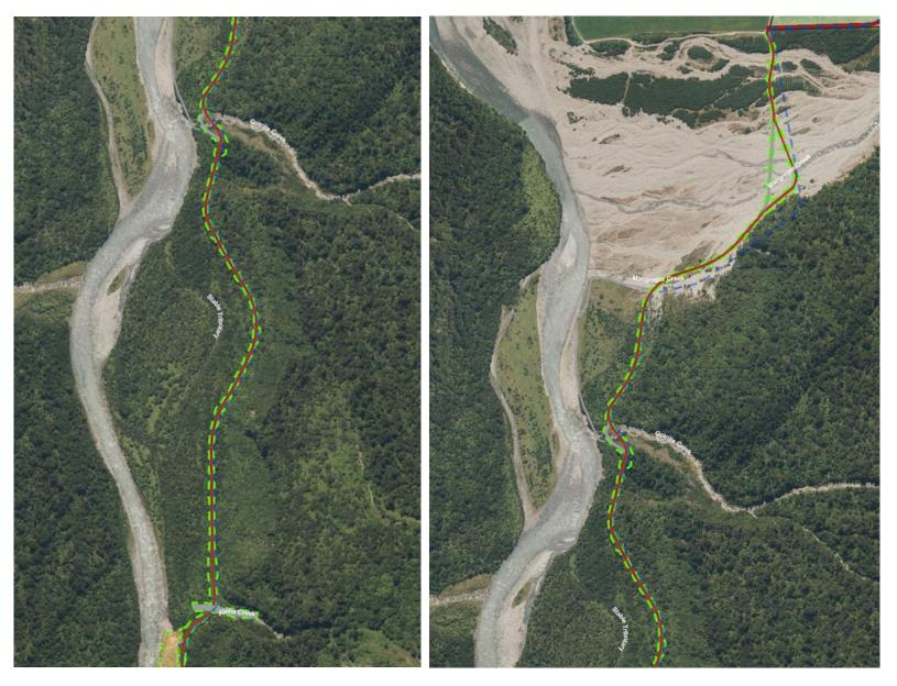
**Figure 4.** Access road north of Power Station (left image) and portion south of Macgregor Creek (right image). The access road is shown by the red line, with the total disturbance boundary shown by the green dotted line.
