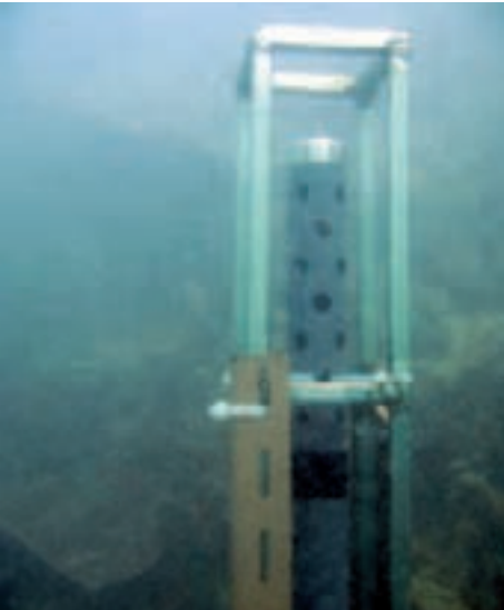
Figure 17. Left: deployed YSI turbidity sensor. Right: Time series of turbidity measurements.
