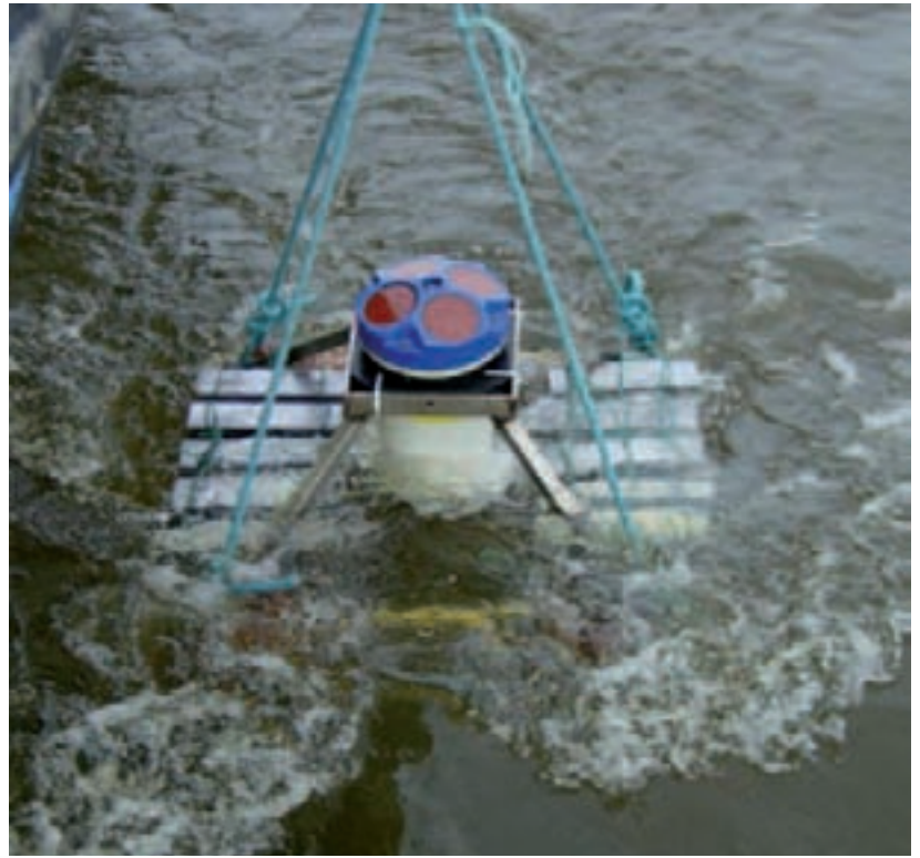
Figure 19. An Acoustic Doppler Current Profiler mounted on a stainless steel frame and about to be deployed on the seabed.
