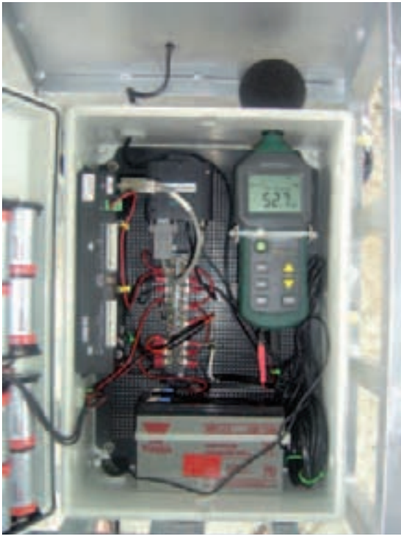
Figure 18. A noise meter, built into a switch box.
