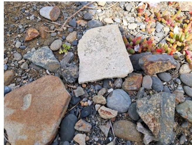
Photo 11. A fragment of fibre board (suspected ACM) found on the east bank.
