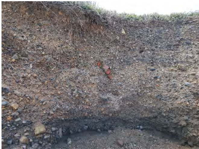
Photo 18. Example of fill contents in the exposed bank.
