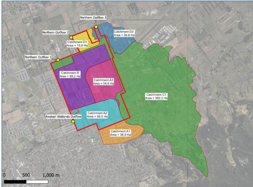
[27D] Following development within A2 of the western catchment, the consent holder shall ensure that no further stormwater flow from the western catchment within the Sunfield development (A3) enters the McLennan Dam until the McLennan Dam is upgraded to meet the required standards of New Zealand Building (Dam Safety) Regulations 2022 for a High Potential Classification dam for the entire western catchment (A1, A2 and A3), to the satisfaction of Council.
