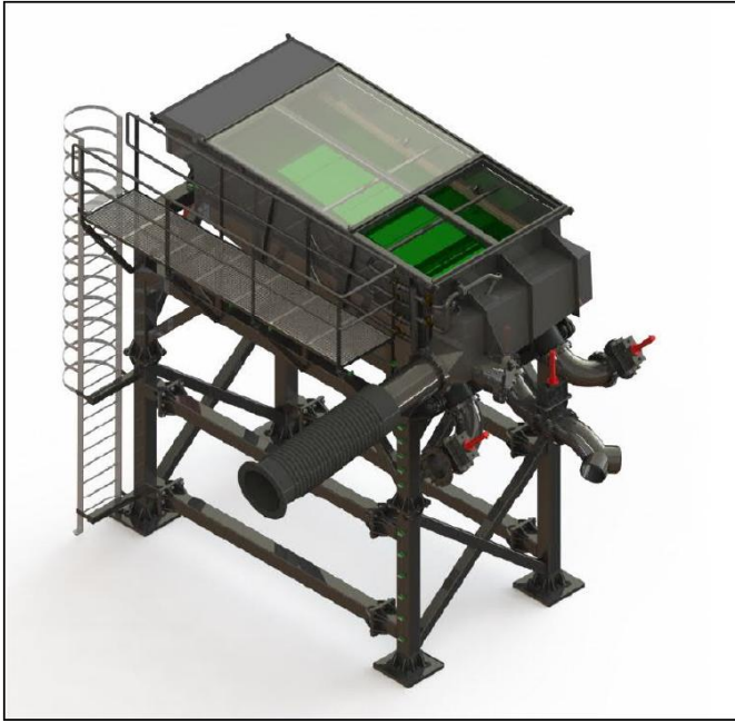
Figure Ten: 3 D Plan of sand ‘screening deck’ on the William Fraser .
