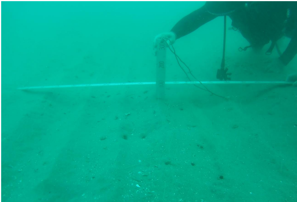
Figure Nine: 80-100mm deep Dredge Track 5 Minutes Post Dredge.
