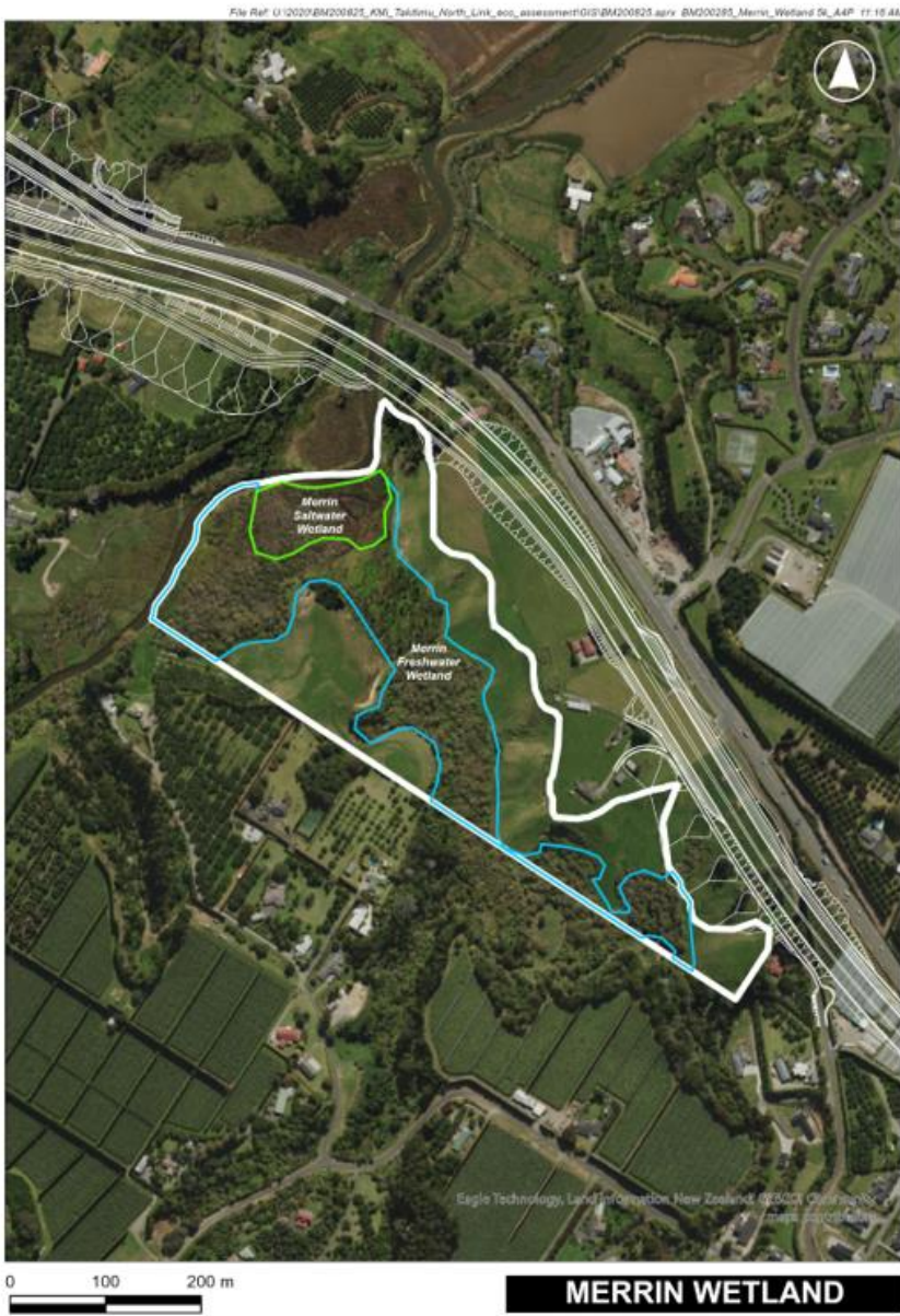
Indicative extent of Merrin Wetland restoration (white outline), freshwater wetland (blue outline/fill), saltmarsh wetland (green outline/fill).
